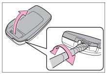
Remove the depleted battery.
