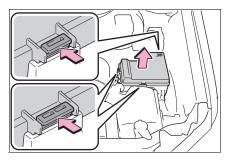
Engine compartment: type B fuse box
