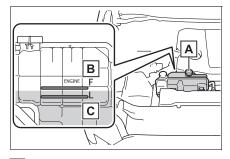
A Engine coolant reservoir cap
