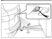
This light's usage for Trailer Backup Guide is controlled by the Trailer Backup Guide system and the driver does not need to activate the light separately.
