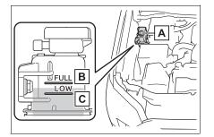
A Power control unit coolant reservoir cap
