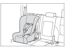
Run the seat belt through the 4 child restraint system and insert the plate into the buckle. Make sure that the belt is not twisted.
