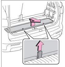
Adjustable deck board The position of the deck board can be changed.
