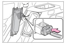
Install the air intake vent cover.
