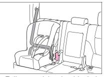
5 Fully extend the shoulder belt and allow it to retract to put it
