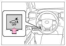
When the Parking Support Brake is disabled, the PKSB OFF indicator ( $\rightarrow$ P.89) illuminates.
