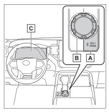
A "DAC/CRAWL" switchB Mode select switch
