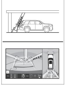
Visually check the surroundings and the area behind the vehicle. In the case shown below, the truck appears to be outside of the estimated course lines and the vehicle does not look as if it hits the truck. However, the rear body of the truck may actually cross over the estimated course lines. In reality if you back up as guided by the estimated course lines, the vehicle may hit the truck.
