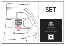
A "Operate Cruise switch or Accelerator Pedal to Resume"
