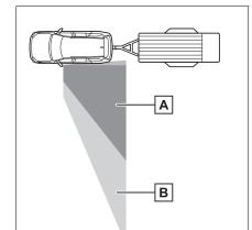
The area able to be seen changes depending on the camera angle adjustments.
