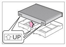
Checking interval Inspect and replace the air conditioning filter according to the maintenance schedule. In dusty areas or
