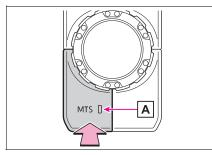
2 Select the Multi-terrain Select modes on the multi-information display while turning the mode select switch left and right.
