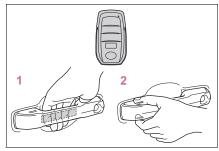
Grip the driver's door handle to unlock the door. Holding the driver's door handle for approximately 2 seconds unlocks all the doors. Grip front passenger door handle
