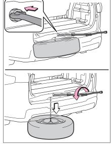
4 After the tire is lowered completely to the ground, remove the holding bracket.
