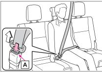
2 Insert the mechanical key (→P.110) or plate B into the notch of buckle and remove the belt.
