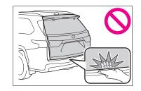
Use caution when using the back door closer as it still operates when the power back door system is canceled.
