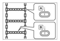
A Side chain (0.2 in. [5 mm] in diameter)
