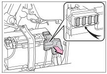
3 Remove the fuse with the pullout tool.Only type A fuse can be
