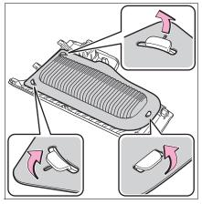
**5** Remove the dust and sand from the filter.
