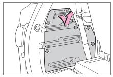
Remove the positive (+) battery terminal cover.
