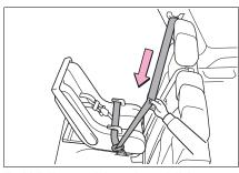
5 While pushing the child restraint system down into the rear seat, allow the shoulder belt to retract until the child restraint system is securely in place.
