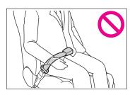
The SRS front passenger airbag also deploys with considerable force, and can cause death or serious injury especially if the front passenger is very close to the airbag. The front passenger seat should be as far from the airbag as possible with the seatback adjusted, so the front passenger sits upright.
