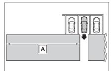
The buzzer can alert for faster vehicles approaching from farther away.
