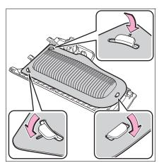
Make sure that the filter is not crooked or deformed when installing it.
