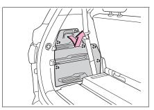
2 After removing the cover, pull the lever to unlock the fuel door and it will be ready to open as usual.
