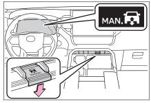
The height can be adjusted by pressing the height control switch.
