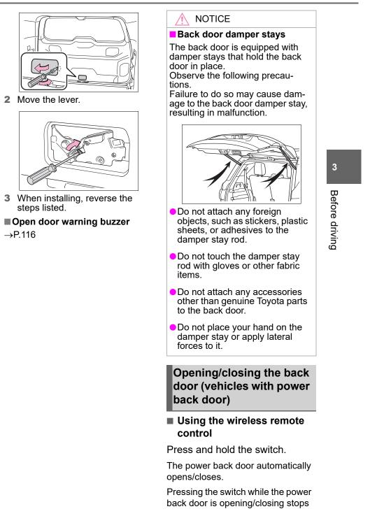
the operation. When the switch is pressed and held again during the halted operation, the back door will perform the reverse operation.
