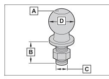
A Trailer ball load rating Matches or exceeds the gross trailer weight rating of the trailer.
