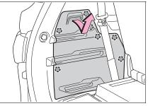
**2** Unhook the belt, and loosen and remove the jack.
