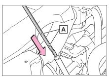
5 Holding a rag under the end, pull the dipstick out and check whether the oil level is above low level mark.
