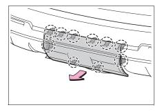
■ When installing the cover Be sure to install the 10 claws.
