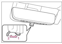
**1** Digital mirror mode Displays an image of the area behind the vehicle.
