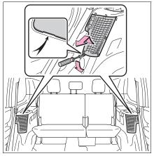
3 Vehicles with third seat (power type): Remove the third seatback folding/returning switch connector.
