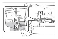
A Intercooler coolant reservoir cap
