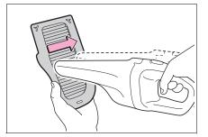
6 Hold the filter to the light and check if it is not clogged.
