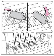
Remove the support parts: To remove the support parts, push the claw and lift it up.
