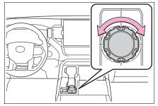
Front-wheel drive control switch is in "4L"
