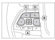
A Scroll the screen<sup>\*</sup>/switch the display<sup>\*</sup>/move the cursor
