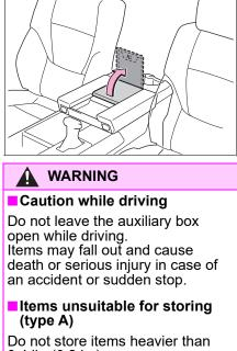
0.4 lb. (0.2 kg). Doing so may cause the auxiliary box to open and the items inside may fall out, resulting in an accident. Luggage compartment features
