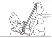
4 Fully extend the shoulder belt and allow it to retract to put it in lock mode. In lock mode, the belt cannot be extended.
