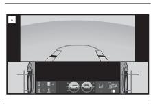
When the under vehicle terrain view and side view screens are touched, each of the display sizes can be changed.
