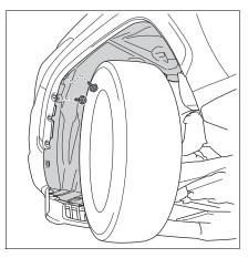
2 Open the fender liner and turn the bulb base counterclockwise.
