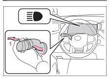
1 With the headlights on, push the lever away from you to turn on the high beams.
