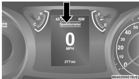
3.5 Inch Instrument Cluster Display Location
