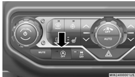
Stop/Start OFF Switch
