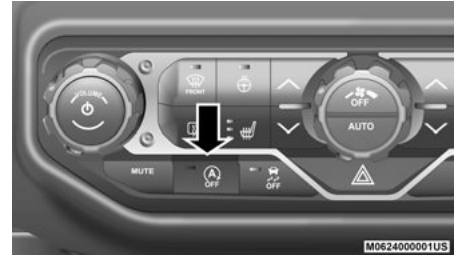
Stop/Start OFF Switch
