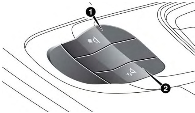
Courtesy Light Switches
