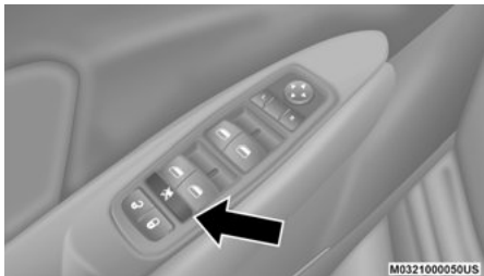
Window Lockout Switch
