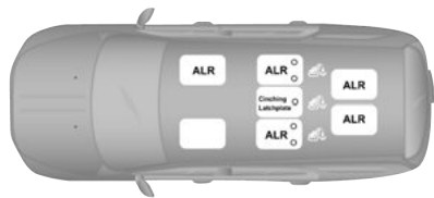
ALR — Switchable Automatic Locking Retractor (Third Row Shown — If Equipped)
