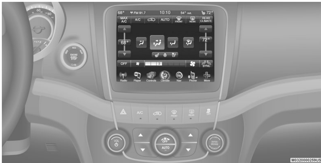
Uconnect 3/3 NAV Automatic Tri-Zone Temperature Controls
