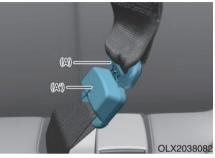
2.Insert the tongue plate (A) into the buckle (A') until an audible "click" is heard, indicating the latch is locked. Make sure the belt is not twisted.
