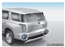
The rear radars are located inside the rear bumper for detecting the side and rear areas. Always keep the rear bumper clean for proper operation of the system.
