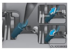
3. Pull out the tongue plate (B) from the pocket. Pull the tongue plate (B) and insert it into the buckle (B') until an audible "click" is heard, indicating the latch is locked. Make sure the belt is not twisted.
