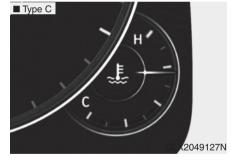
This gauge indicates the temperature of the engine coolant when the ignition switch is in the ON position.
