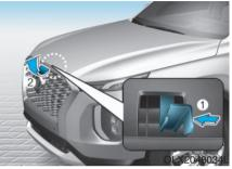
3. Go to the front of the vehicle, raise the hood slightly, push up the secondary latch (1) inside of the hood center and lift the hood (2). After it has been raised about halfway, it will raise completely by itself.
