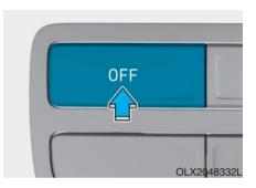
Push the OFF button to turn the rear climate control system off.
