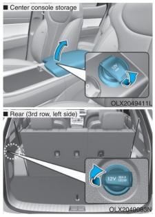
The power outlet is designed to provide power for mobile telephones or other devices designed to operate with vehicle electrical systems. The devices should draw less than 180 W with the engine running.
