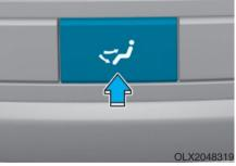
You can select the direction of the air flow through the ventilation system.
