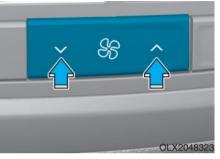
2. The fan speed can be set to the desired speed by pushing the fan speed control button. The higher the fan speed is, the more air is delivered. Pressing the OFF button turns off the fan.
