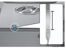
6. Pull the dipstick out again and check the level. The level should be between F and L.
