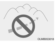
Do not drive across the contour of steep hills. A slight change in the wheel angle can destabilize the vehicle, or a stable vehicle may lose stability if the vehicle stops its forward motion. Your vehicle may roll over and lead to a serious injury or death. Driving through water
