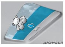
If the sunroof senses any to an obstacle while it is closing automatically, it will reverse direction then stop to allow the object to be cleared.
