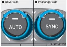
2. To select a different set point, turn the temperature control knob to the desired temperature. If the temperature is set to the lowest setting (Lo), the air conditioning system will operate continuously. After the interior has cooled sufficiently, adjust the knob to a higher temperature set point whenever possible. To turn the automatic operation off, select any button of the following:
