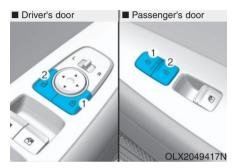
The driver side and front passenger side door armrest is equipped with a central door lock switch. The lock button is indicated by a (1) symbol. The unlock button is indicated by a (1) symbol.
