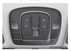
If your vehicle is equipped with a sunroof, you can slide or tilt your sunroof with the sunroof control lever located on the overhead console.
