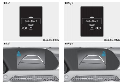
If the risk of collision is detected while the RCCW is generated, brake is controlled. The instrument cluster will inform the driver of the brake control. If the rear view monitor system is in activation, a message will also appear on the infotainment screen.
