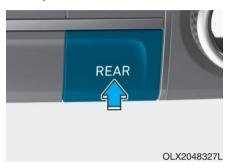
1. Press the rear climate control button of the front climate control system.
