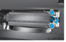
3. Remove the climate control air filter case while pressing the lock on right side of the cover.
