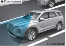
In order for the FCA system to operate properly, always make sure the sensor cover or sensor is clean and free of dirt, snow, and debris. Dirt, snow, or foreign substances on the sensor cover or sensor may adversely affect the sensing performance of the sensor.
