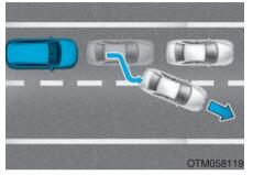
• When driving in stop-and-go traffic, and a vehicle in front of you merges out of the lane, the system may not immediately detect the new vehicle that is now in front of you. In this case, you must maintain a safe braking distance, and if necessary, depress the brake pedal to reduce your driving speed in order to maintain a safe distance.
