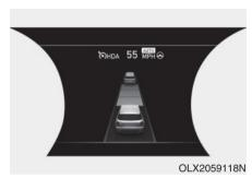
When the highway speed limit changes, the set speed automatically changes to the changed speed limit.
