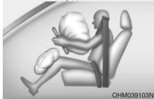
Upon deployment, tear seams molded directly into the pad covers will separate under pressure from the expansion of the air bags. Further opening of the covers allows full inflation of the air bags.
