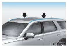
If your vehicle comes equipped with roof side rails, then roof rack crossbars can be installed on top of your vehicle.
