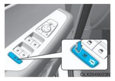
The driver can disable the power window switches on the rear passenger doors by pressing the power window lock switch.
