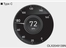
The speedometer indicates the speed of the vehicle and is calibrated in miles per hour (MPH) and/or kilometers per hour (km/h).
