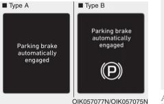
Parking brake automatically engaged
