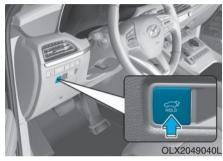
Power liftgate button Press the power liftgate button for approximately one second.
