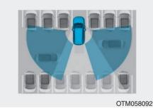
The Rear Cross-Traffic Collision Warning (RCCW) system uses radar sensors to monitor the approaching cross traffic from the left and right side of the vehicle when your vehicle is in reverse.
