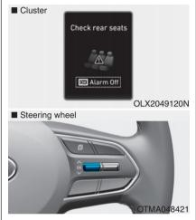
If you do not want to use the Rear Occupant Alert (ROA) system, press OK button on the steering wheel when the 1st alert is displayed on the cluster. Doing so will deactivate the 2nd alert once. (if equipped)
