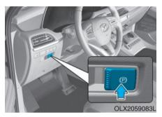
To release the EPB (Electronic Parking Brake):
