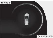
• If the driver turns off the engine when the sunroof is not fully closed, the warning chime will sound for approximately 3 seconds and the sunroof open warning will appear on the cluster LCD display.
