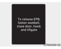
To release EPB, fasten seatbelt, close door, hood and liftgate
