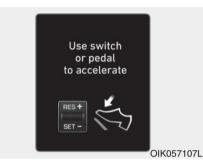
If you push the smart cruise control toggle switch (RES+ or SET-) while Auto Hold and smart cruise control is operating the Auto Hold will be released regardless of accelerator pedal operation and the vehicle will start to move. The AUTO HOLD indicator changes from green to white.
