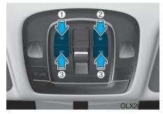
Front Room Lamp (1) ( 亦): Press the button to turn the front and rear room lamps on or off. Front Door Lamp (2) (  $\overline{\square}$  ):
