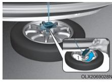
Draw out the retainer guide (1) through the center hole of the spare tire. To store the spare tire:
