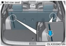
4. Pull up the seatback recline lever, then fold the seat toward the front of the vehicle.
