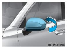
To fold the side view mirrors, grasp the housing of the mirror and then fold it inwards.
