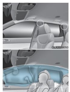
Curtain air bags are located along both sides of the roof rails above the front and rear doors. They are designed to help protect the heads of the front seat occupants and the rear outboard seat occupants in certain side impact collisions.
