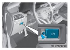
To apply the EPB (Electronic Parking Brake): 1. Depress the brake pedal. 2. Pull up the EPB switch. Make sure the Parking Brake Warning Light comes on.
