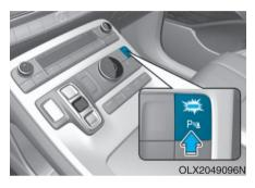
Push the button to turn OFF the Reverse Parking Distance Warning system. The indicator light on the button will turn on.
