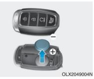
If the Smart Key is not working properly, try replacing the battery with a new one.
