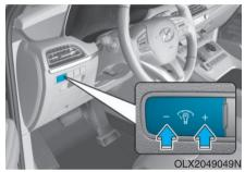
When the vehicle's position lights or headlights are on, press the illumination control button to adjust the brightness of the instrument panel illumination.
