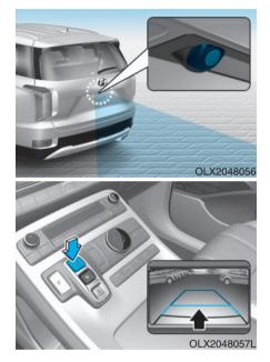
The Rear View Monitor will activate when the engine is running and the shift button is in the R (Reverse) position. This is a supplemental system that helps provide a view of the area behind the vehicle through the infotainment system screen while the vehicle is in the R (Reverse) position.
