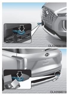
If towing is necessary, we recommend you have it done by an authorized HYUNDAI dealer or a commercial tow truck service. If towing service is not available in an emergency, your vehicle may be temporarily towed using a cable or chain secured to the emergency towing hook at the front (or rear) of the vehicle.
