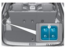
Push the 3rd row seat back folding switch (1) located on the left side of the cargo area. (L : Left seatback folding/unfolding, R : Right seatback folding/unfolding)
