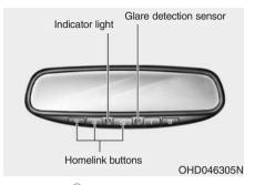
HomeLink<sup>®</sup> Wireless Control System Your new mirror comes with an integrated HomeLink Universal Transceiver, which allows you to program the mirror to activate your garage door(s), estate gate, home lighting, etc. The mirror actually learns the codes from your various existing transmitters.
