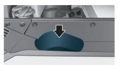
Step back while the pressure is released from the cooling system. When you are sure all the pressure has been released, press down on the cap, using a thick towel, and continue turning counterclockwise to remove it.
