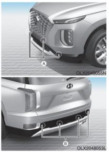
[A] : Front Sensor, [B] : Rear Sensor
