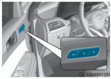
The Driver Position Memory System is provided to store and recall the following memory settings with a simple button operation.
