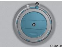
The rear passengers can adjust the direction of air flow from the rear vents on the headliner.
