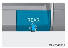
1. Press the rear climate control button of the front climate control system.
