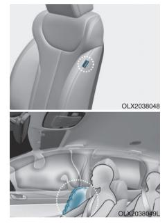
Your vehicle is equipped with a side air bag in each front seat. The purpose of the air bag is to provide the vehicle's driver and the front passenger with additional protection than that offered by the seat belt alone. The side air bags are designed to deploy during certain side impact collisions, depending on the crash severity.
