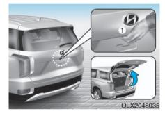
Before attempting to open the liftgate, make sure the vehicle is in P (Park). To open the liftgate, perform one the following:
