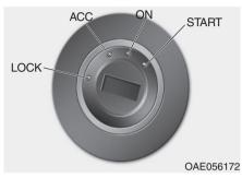
Whenever the front door is opened, the ignition switch will illuminate, provided the ignition switch is not in the ON position. The light will go off immediately when the ignition switch is turned on or go off after about 30 seconds when the door is closed. (if equipped)
