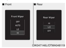
This indicator displays which wiper speed is selected using the wiper control.
