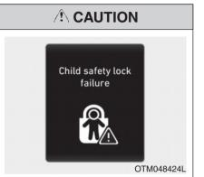
If the Electronic child safety lock system is not operated when pushing the Electronic child safety lock switch, the message is displayed and the alarm will sound.
