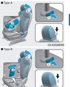
To reinstall the head restraint:
