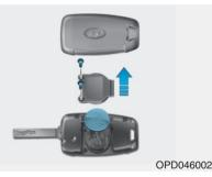
If the remote key is not working properly, try replacing the battery with a new one.
