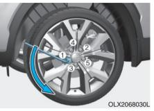
Loosen the wheel lug nuts counterclockwise one turn each in the order shown above, but do not remove any lug nuts until the tire has been raised off of the ground.
