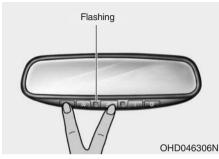
1. When programming the buttons for the first time, press and hold the left and center buttons (⊉, <u>1</u>) simultaneously for approximately 20 seconds until the indicator light begins to flash. (This procedure erases the factory-set default codes. Do not perform this step to program additional hand-held transmitters.)
