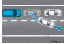
When driving in stop-and-go traffic, and a vehicle in front of you merges out of the lane, the FCA system may not immediately detect the new vehicle that is now in front of you. In this case, you must maintain a safe braking distance, and if necessary, depress the brake pedal to reduce your driving speed in order to maintain a safe distance.
