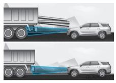
• Detecting the vehicle in front of you If the vehicle in front of you has cargo that extends rearward from the cab, or when the vehicle in front of you has higher ground clearance, additional special attention is required. The FCA system may not be able to detect the cargo extending from the vehicle. In these instances, you must maintain a safe braking distance from the rearmost object, and if necessary, depress the brake pedal to reduce your driving speed in order to maintain distance.
