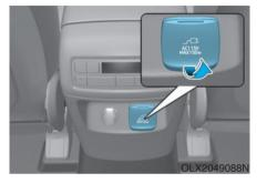
The AC inverter supplies 115V/150W electric power to operate electric accessories or equipments.
