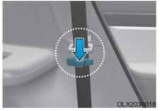
Locate the seatbelt webbing in the guide before folding down the seatback to avoid the seatbelt system interfering with the seatback.
