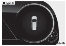
This warning is displayed if you turn off the engine when any window is open.
