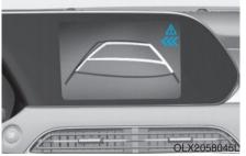
If the vehicle detected by the sensors approaches from the rear left/right side of your vehicle, the warning chime will sound, the warning light on the outer side view mirror will blink and a warning will appear on the LCD display. If the rear view monitor system is in activation, a warning will also appear on the infotainment system screen.
