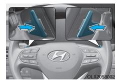
The paddle shifter is available when the gear is in the D (Drive) position. Pull the [+] or [-] paddle shifter once to shift up or down one gear and the system changes from automatic shift mode to manual shift mode.
