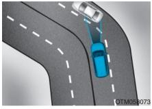
The FCA system may recognize a vehicle in the next lane when driving on a curved road.
