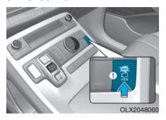
The Surround View Monitoring system can assist in parking by allowing the driver to see around the vehicle.
