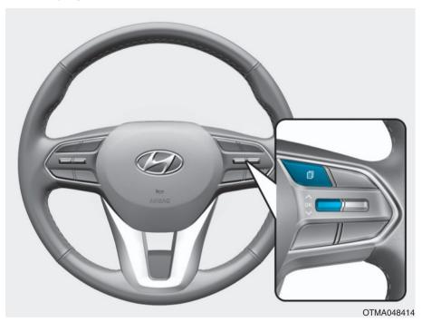
The LCD display modes can be changed by using the control buttons.
