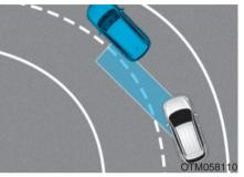
The BCW and BCA systems may not operate properly when driving on a curved road. In certain instances, the system may recognize a vehicle in the same lane.
