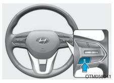
When the Smart Cruise Control system is ON, you can set and maintain the distance from the vehicle ahead of you without pressing the accelerator or brake pedal. Each time the button is pressed, the vehicle to vehicle distance changes as follows:
