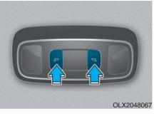
Rear Room Lamp ( ァ 도): Press either buttons to turn the room lamp on or off.
