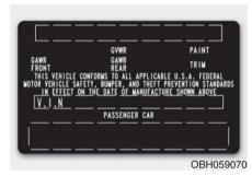
The total weight of the vehicle, including all occupants, accessories, cargo, and trailer tongue load must not exceed the Gross Vehicle Weight Rating (GVWR) or the Gross Axle Weight Rating (GAWR). To find out the actual loads on your front and rear axles, you need to go to a weigh station and weigh your vehicle. Be sure to spread out your load equally on both sides of the centerline.
