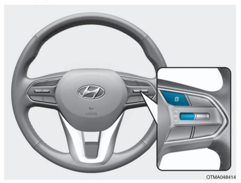
The LCD display modes can be changed by using the control buttons.
