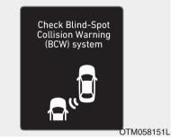
Check Blind-Spot Collision Warning (BCW) system
