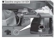
The engine number is stamped on the engine block as shown in the drawing.
