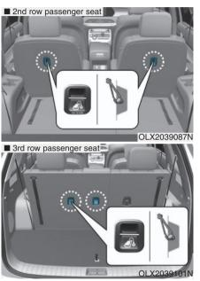
First secure the child restraint with the LATCH lower anchors or the seat belt. If the child restraint manufacturer recommends that the top tether strap be attached, attach and tighten the top tether strap to the top tether strap anchor. Child restraint hook holders are located on the rear of the seatbacks.
