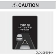
If the vehicle ahead (vehicle speed: less than 20 mph (30 km/h)) moves to the next lane, the warning chime will sound and a message "Watch for surrounding vehicles" will appear. Adjust your vehicle speed for vehicles or objects that can suddenly appear in front of you by depressing the brake pedal.
