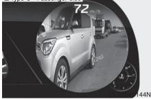
BVM (Blind-spot View Monitor) system displays the driver-side or passenger-side rear areas in the cluster when the system is activated.
