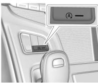
The automatic engine Stop/Start feature can be disabled and enabled by pressing A. Auto Stop/Start is enabled each time you start the vehicle.
