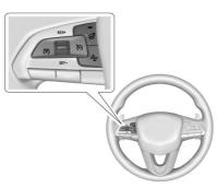
(S) : Press to turn the system on or off. The indicator turns white on the instrument cluster when ACC is turned on.
