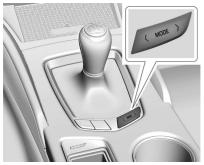
Driver Mode Control Switch for Manual Transmission
