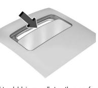
Dirt and debris may collect on the sunroof seal or in the track. This could cause an issue with sunroof operation or noise. It could also plug the water drainage system. Periodically open the sunroof and remove any obstacles or loose debris. Wipe the sunroof seal and roof sealing area using a clean cloth, mild soap, and water. Do not remove grease from the sunroof.
