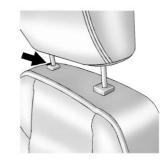
To lower the head restraint, press the button, located on the top of the seatback, and push the head restraint down. Try to move the head restraint after the button is released to make sure that it is locked in place.
