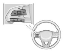
(S): Press to turn cruise control on and off. A white indicator light appears in the instrument cluster when cruise control is turned on.
