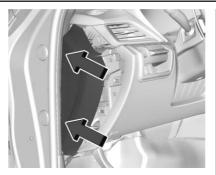
To install the end cover, insert the tabs on the back of the cover into the slots in the instrument panel at the points shown. Align the clips with the slots in the instrument panel, and press the cover into place.
