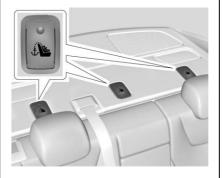
The top tether anchors are behind the rear seat, on the filler panel. Open the covers to access the anchors. Be sure to use an anchor located directly behind the seating position where the child restraint will be placed.
