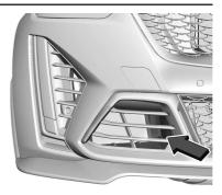
3. Front Brake Cooling Duct
