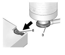
5. Slide the base of the tire sealant canister (3) into the slot on the top of the compressor (6) to hold it upright.
