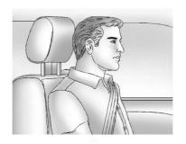
If equipped with base seats, adjust the head restraint so that the top of the restraint is at the same height as the top of the occupant's head. This position reduces the chance of a neck injury in a crash.
