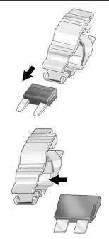
3. Use the fuse puller to remove the fuse from the top or side, as shown above.
