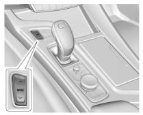
Driver Mode Control Switch for Automatic Transmission
