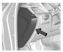
To access the fuses, remove the end panel by gently prying with a plastic tool near each clip, beginning at the point shown.
