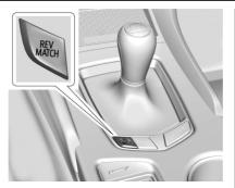
The system is activated and deactivated by pressing the ARM switch on the center console. The system must be activated with each new ignition cycle. If ARM is deactivated, the system will still perform rev matching for upshifts.
