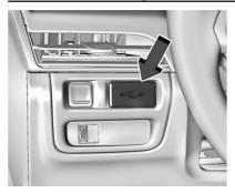
The PDR records video, audio, and vehicle data. This data is stored on a removable SD card located to the left of the steering wheel.
