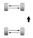
Use this rotation pattern if the vehicle has different size tires on the front and rear.
