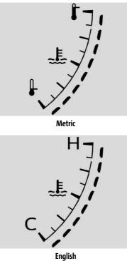
This gauge measures the temperature of the vehicle's engine.
