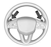
If equipped, vehicles with Tap Shift have controls on the back of the steering wheel to manually shift the automatic transmission.
