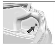
Insert an SD card into the card reader in the trunk. Disable the system from the playback screen before removing the SD card from the reader. Do not remove the card while recording is enabled. This could corrupt the video file and/or the SD card.
