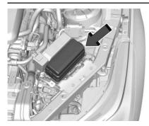
Lift the fuse block cover to access the fuses. The vehicle may not be equipped with all of the fuses and relays shown.
