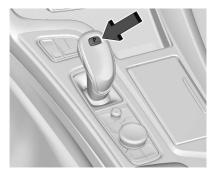
**P** : This position locks the drive wheels. Use P (Park) when starting the engine to prevent the vehicle from moving easily.
