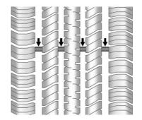
Treadwear indicators are one way to tell when it is time for new tires. Treadwear indicators appear when the tires have only 1.6 mm (1/16 in) or less of tread remaining. See *Tire Inspection*  $\Rightarrow$  339 and *Tire Rotation*  $\Rightarrow$  340.
