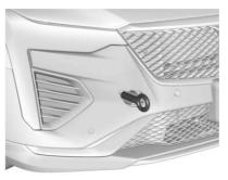
The vehicle is equipped with a tow eye. Only use the tow eye to pull the vehicle onto a flatbed car carrier from a flat road surface. Do not use the tow eye to pull the vehicle from snow, mud, or sand. The tow eye is located under the carpet in the trunk.
