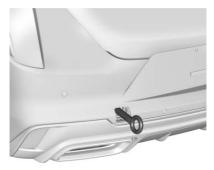
If equipped, carefully open the cover by using the small notch that conceals the rear tow eye socket. Install the tow eye into the socket and turn it until it is fully tightened. When the tow eye is removed, reinstall the cover with the notch in the original position.
