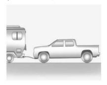
Only dinghy tow four-wheel-drive vehicles with a two-speed transfer case that have an N (Neutral) and a 4 \$\dpsi\$ (Four-Wheel Drive Low) setting.
