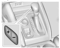
Range Selection mode helps control the vehicle's transmission and vehicle speed while driving downhill or towing a trailer by letting you select a desired range of gears.
