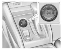
If equipped, the transfer case controls are used to shift into and out of four-wheel drive.
