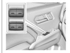
Power windows work when the vehicle is on, in accessory mode, or when Retained Accessory Power is active. See *Retained Accessory Power (RAP)*
