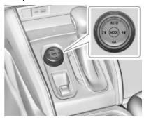
If equipped, the transfer case controls are used to shift into and out of four-wheel drive.
