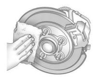
8. Remove any rust or dirt from the wheel bolts, mounting surfaces, and spare wheel.
