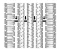
Treadwear indicators are one way to tell when it is time for new tires. Treadwear indicators appear when the tires have only 1.6 mm (1/16 in) or less of tread remaining. See *Tire Inspection* ⇔ 277 and *Tire Rotation* ⇔ 277.
