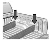
The board closest to the cab should be cut to an approximate length of 117 cm (46 in). The board closest to the tailgate should be cut to an approximate length of 150 cm (59 in).
