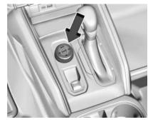
To activate each mode, turn the MODE knob on the center console in either direction.
