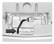
Go to the front of the vehicle and locate the secondary release lever under the front center of the hood. Push the secondary hood release lever to the right to release.
