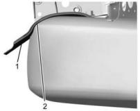
7. Make sure the tire is stored securely and flush in the radius (2) of the spare tire support bracket (1). Push, pull, and then try to turn the tire. If the tire moves, use the wheel wrench to tighten the cable. Repeat this tightness check procedure when checking the spare tire pressure according to the scheduled maintenance information or any time the spare tire is handled due to service of other components.
