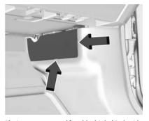
The instrument panel fuse block is behind a side trim panel. Unclip the sides of the trim, then pull the cover away from the trim panel to access the fuse block.
