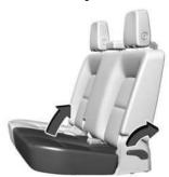
To fold the seat, lift the lever fully and pull the seat cushion up.
