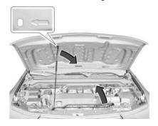
Lift the hood only enough to release the hood prop rod from its retainer, and insert it into the slot marked with an arrow on the underside of the hood. Lifting the hood too far may disengage the parts adjacent to the hinges.
