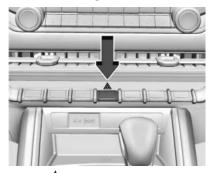
Press the Abutton to make the front and rear turn signal lights flash on and off. This warns others that you are having trouble. Press again to turn the flashers off.
