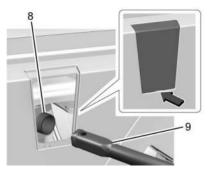
2. Remove the hoist shaft access hole cover on the bumper.
