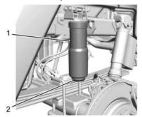
Jounce Control Dampers (1), if equipped, help with spirited driving. They compress when the suspension moves upward enough to engage the dampers. This will result in a slight clicking sound as the axle or control arms contact the pad of the jounce control damper. This noise is normal and is part of the operation of the system. Over time, the plastic caps (2) on the jounce control dampers will wear and should be replaced.
