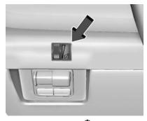
Rotate this thumbwheel  $\mathcal{E}_3^{\mathfrak{Q}}$  up or down to adjust the brightness of all illuminated controls. The thumbwheel is on the instrument panel to the left of the steering wheel.
