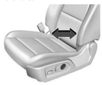
If equipped, press and hold the front or rear of the control to increase or decrease lumbar support.
