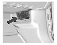
There is a cover on the instrument panel fuse block. Press the clips on the side to remove the cover.
