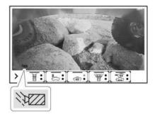
Touch the symbol on the lower-left of the infotainment display to activate the washer
