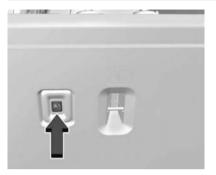
The second row seat can also be moved for third row exit by pressing the switch on the seatback of the second row seat.
