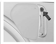
3. Press the button to manually close the charge port door.
