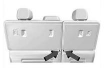
Use the emergency pull strap only if the vehicle loses power. The emergency strap can be pulled from the second or third row seat to incline the seat forward for exit of a person in the third row. To fold the second row seatbacks by using the emergency pull strap:
