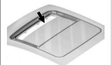
Dirt and debris may collect on the sunroof seal or in the track. This could cause an issue with sunroof operation or noise. It could also plug the water drainage system.
