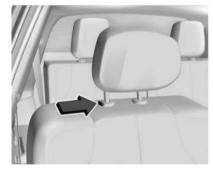
To lower the head restraint, press the button, located on the top of the seatback, and push the head restraint down. After releasing the button, ensure the head restraint locks in place and is unable to move up or down.
