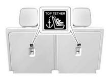
The top tether anchors for each rear seating position are on the back of the rear seatback. Be sure to use an anchor located directly behind the seating position where the child restraint will be placed.
