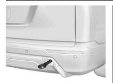
2. Install the tow eye into the socket and turn it until it is fully tightened. When the tow eye is removed, reinstall the cover with the notch in the original position.
