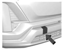
1. Carefully open the cover on the fascia by using the small notch that conceals the tow eye socket.
