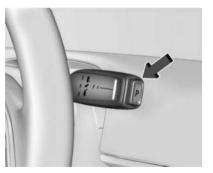
The vehicle uses an electric drive unit. The shift pattern is displayed on the front of the shift lever. The selected gear position will illuminate red on the shift lever, while all others will be displayed in white. If the shift is not immediate, as in very cold conditions, the indicator on the shift switch may blink until it is fully engaged.
