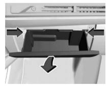
2. Press the sides of the glove box bin inward to clear the stoppers and turn downward to lower the bin.
