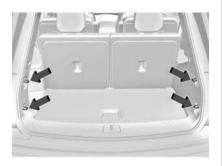
The vehicle has four cargo tie-downs in the rear compartment.
