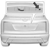
To access the liftgate key lock cylinder, insert the mechanical key into the cylinder and turn to unlock. See *Keys* r > 6.
