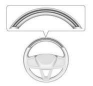
The steering wheel light bar and instrument cluster light provide the following important information about Super Cruise operation:
