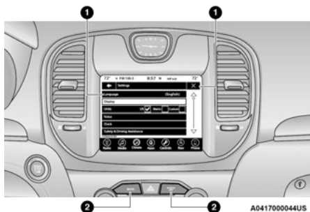
Uconnect 4C/4C NAV With 8.4-inch Display Buttons On The Touchscreen And Buttons On The Faceplate
