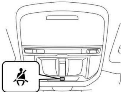
Front passenger's warning light
