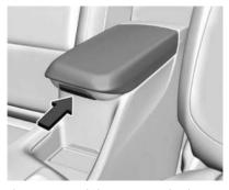
The center console has storage under the armrest. Push the latch and lift to open.
