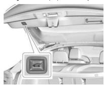
Press on the bottom edge of the liftgate to the left of the latch to close.
