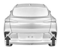
The bulbs are accessible from the underside of the vehicle.
