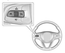
**RES+:** If cruise control is already engaged, press the thumbwheel up to increase the set speed. If there is a set speed in memory, press up briefly to engage cruise control at the previous set speed.
