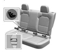
The outboard lower anchors are behind the vertical openings in the seat trim.
