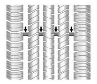
Treadwear indicators are one way to tell when it is time for new tires. Treadwear indicators appear when the tires have only 1.6 mm (1/16 in) or less of tread remaining. See *Tire Inspection* ⇔ 229 and *Tire Rotation* ⇔ 230.
