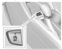
If equipped, the automatic engine stop/start feature can be disabled and enabled by pressing the switch with the  $^{(A)}_{\rm DF}$  symbol. Auto Stop is enabled each time you start the vehicle.
