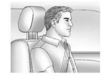
Adjust the head restraint so that the top of the restraint is at the same height as the top of the occupant's head. This position reduces the chances of a neck injury in a crash.
