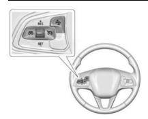
ress to turn the ACC system on or off. The indicator light turns white on the instrument cluster when ACC is turned on.
