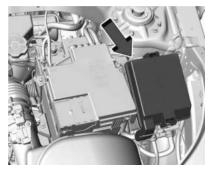
To remove the fuse block cover, squeeze the clip and lift it up.  $\label{eq:cover_squeeze}$
