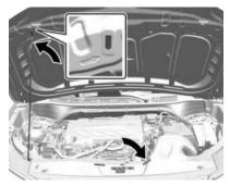
Lift the hood and release the hood prop from its retainer, above the radiator.
