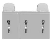
The top tether anchors for each rear seating position are on the back of the rear seatback. The rear compartment storage panel/cover
