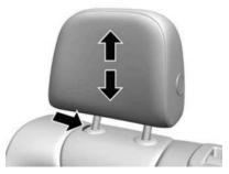
To lower the head restraint, press the button on the top of the seatback and push the head restraint down. After releasing the button, ensure the head restraint locks in place and is unable to move up or down.
