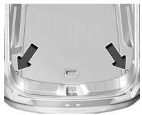
The vehicle may be equipped with two cargo tie-downs in the rear compartment.
