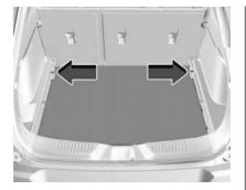
The cargo management system has an angle adjustment to secure the load floor while removing stored items.
