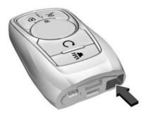
2. Insert a flat, thin object and remove the back cover.
