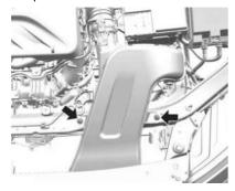
Remove the two push pins.
