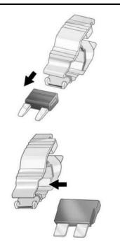
3. Use the fuse puller to remove the fuse from the top or side, as shown above.
