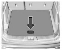
2. Lift the load floor by the handle.
