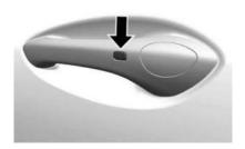
The remote key must be within 1 m (3 ft) of the liftgate or door being opened. Press the button on the door handle to open. See *Remote Key Operation*  $\ \ \ \ \ \ \ \ \ \$  9.
