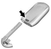
Press the button on the bottom of the remote key to remove the key. Never pull the key out without pressing the button.
