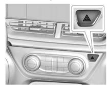
Press the button to make the front and rear turn signal lights flash on and off. This warns others that you are having trouble. Press again to turn the flashers off.
