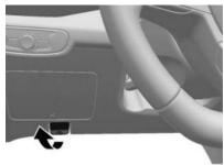
Pull the hood release handle inside the vehicle. It is located on the lower left side of the instrument panel.
