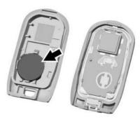
3. Lift the battery with a flat object.
