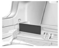
In the rear compartment storage area, the quarter lower storage panel can be removed on the driver side. Lift the load floor to access and pull the panel to remove.
