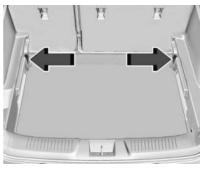
Grasp the load floor by the sides and pull slightly rearward, then slide the load floor into the holding slots. The load floor will stay in the open position.
