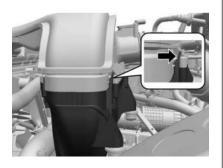
2. Disassemble the duct.
