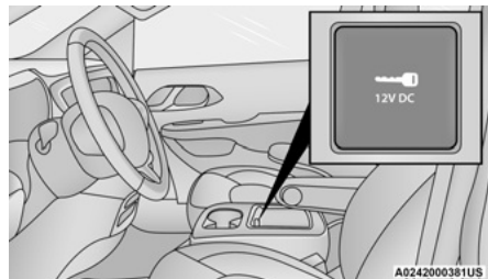
12 Volt Front Power Outlet (In Center Console)
