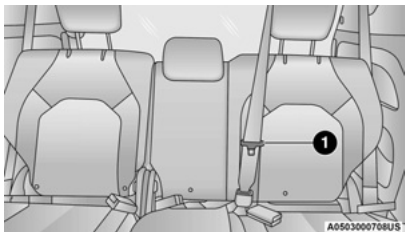
Routing The Rear Seat Belt Latch Plate
