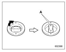
2. Turn the upper knob of each retaining hook (clip) to secure the floor mats in place.
