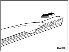
3. Align the claws of the support with the grooves in the rubber and slide the blade rubber assembly into the support until it locks.
