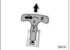
To open the trunk lid from inside the trunk, pull the yellow handle as indicated by the arrow on the handle. This operation unlocks the trunk lid. Then, push up the lid
