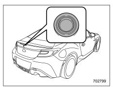
A rear view camera is attached to the trunk lid. When the ignition switch is in the "ON" position and the shift lever (MT models) or select lever (AT models) is set to "R", the rear view camera automatically displays the rear view image behind the vehicle on the center information display.
