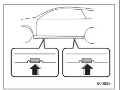
7. Place the jack under the side sill at the front or rear jack-up point closest to the tire to be replaced.
