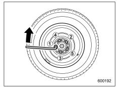
13. Use the wheel nut wrench to securely tighten the wheel nuts to the specified torque, following the tightening order in the illustration.
