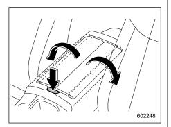
To open the center console, push on the button lightly and it will automatically open.
