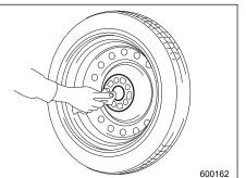
10. Before putting the new tire on, clean the mounting surface of the wheel and hub with a cloth.
