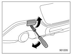
Insert a screwdriver, with its tip covered with tape or a cloth to prevent damage to the bumper, into the cutout of the cover on the rear bumper, pry off the
