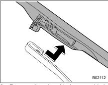
3. Remove the wiper blade assembly by holding its pivot area and pushing it in the direction shown by the arrow.
