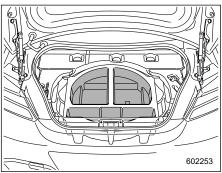
The subfloor storage compartment is located under the floor of the trunk and can be used to store small items. To open the lid, pull the tab or handle up.
