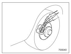
The disc brake pad wear warning indicators on the disc brakes give a warning noise when the brake pads are worn.
