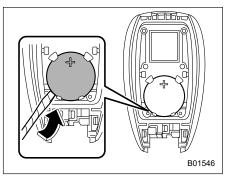
3. Take out the battery using a flat-head screwdriver with vinyl tape or a cloth.
