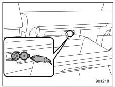
4. Connect the power plug of the air compressor into the accessory power
