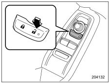
To disable the keyless access function by operating the driver's door, perform the following procedures.
