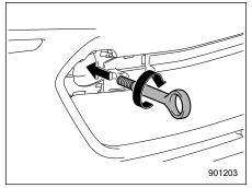
Screw the towing hook into the threaded hole until the threads can no longer be seen.
