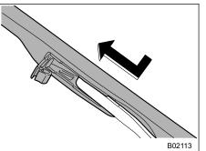
4. When installing the wiper blade assembly, align it with the wiper arm connection part and then slide it in the opposite direction of removal to install.
