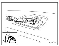
8. Latch the top tether hook onto the tether anchorage that is located behind the rear seat and tighten the top tether firmly. For additional instructions, refer to "Top Tether Anchorages" \$\tilde{F}\$P61.
