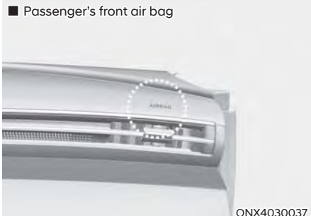
■ Passenger's front air bag
