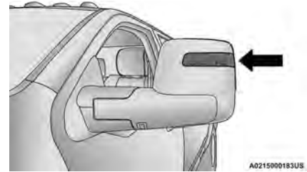
Forward Utility Light
