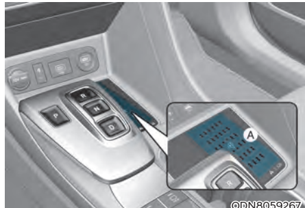
[A] : Wireless Charging Pad (In-vehicle Authentication Pad)
