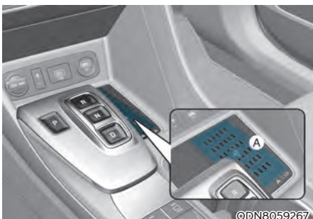
[A] : Wireless Charging Pad (In-vehicle Authentication Pad)
