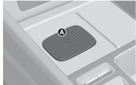
[A] Vehicle authentication pad (wireless charging pad)
