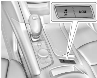
Driver Mode Control Switch
