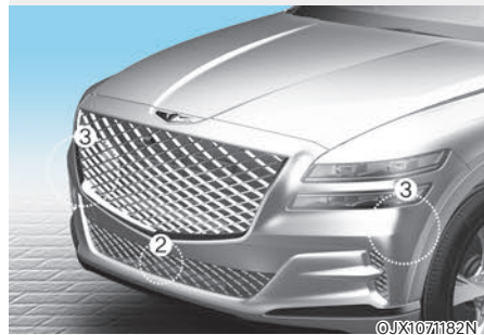
[1]: Front view camera, [2]: Front radar, [3]: Front corner radar (if equipped)
