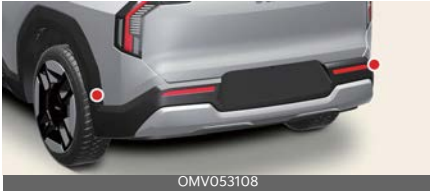
Rear side ultrasonic sensors
