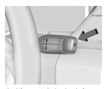
The shift pattern is displayed on the front of the shift lever. The selected gear position will illuminate red on the shift lever, while all others will be displayed in white. If the shift is not immediate, as in very cold conditions, the indicator on the shift switch may blink until it is fully engaged.
