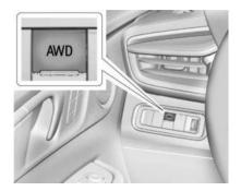
Press the switch to activate the All-Wheel Drive system. The indicator flashes briefly while the system engages and stays lit when the system is active. See All-Wheel-Drive Light ▷ 105.
