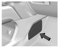
The instrument panel fuse block is inside the center console on the passenger side of the vehicle.
