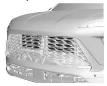
This vehicle may have a shutter system that automatically closes the frontal cooling opening. This system is designed to help improve fuel economy. Ensure the shutter system is clear of any visible debris, snow, or ice.
