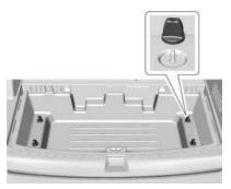
3. Remove the four wing nuts, then remove the cargo management system. See Cargo Management System \$ 84.
