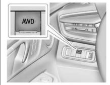
All-Wheel Drive Mode: All-Wheel Drive mode provides drive torque to all four wheels. Select All-Wheel Drive mode to improve traction and control on slippery road surfaces, such as gravel, sand, wet pavement, snow, and ice.
