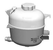
Check to see if coolant is visible in the coolant surge tank. If the coolant inside the coolant surge tank is boiling, do not do anything else until it cools down. If coolant is visible but the coolant level mark is not visible, add a 50/50 mixture of clean, drinkable water and DEX-COOL coolant at the coolant surge tank to the top rib on the middle of the tank, but be sure the cooling system is cool before this is done. See Engine Overheating ♀ 259.
