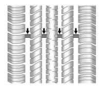
Treadwear indicators are one way to tell when it is time for new tires. Treadwear indicators appear when the tires have only 1.6 mm (1/16 in) or less of tread remaining. See *Tire Inspection* ⇔ 288 and *Tire Rotation* ⇔ 288.
