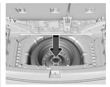
If the vehicle is not equipped with a subwoofer, remove the center wing nut, then remove the spare tire and place it next to the tire being changed.
