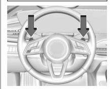
Electronic Range Select, or Manual Mode, allows for the selection of the range of gear positions. Use this mode when driving downhill
