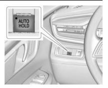
When Automatic Vehicle Hold (AVH) is turned on and the vehicle is braked to a stop, AVH prevents the vehicle from moving during the transition from brake pedal release to accelerator pedal apply. The brakes release when the accelerator pedal is applied. The brakes may also release under other conditions. Do not rely on AVH to hold the vehicle
