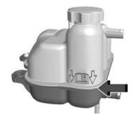
With a cold system, add coolant to the indicated line on the surge tank.
