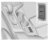
Driver Mode Control Switch for Automatic Transmission
