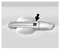
When the doors are locked and the remote key is within 1 m (3 ft) of a door handle, press the lock/unlock button. When unlocking from the driver door, the first press unlocks that door; press again within five seconds to unlock the passenger door and the trunk. See *Remote Key Operation* ♀ 8.
