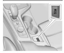
To turn off the Traction Control System, press and release . The Traction Off light displays in the instrument cluster and a message displays in the Driver Information Center. To turn the Traction Control System on again, press and release ♣ See Traction Off Light ♀ 99
