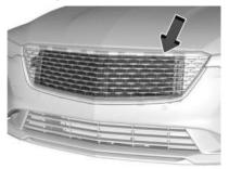
This vehicle may have a shutter system that automatically closes the frontal cooling opening. This system is designed to help improve fuel economy. Ensure the shutter system is clear of any visible debris, snow, or ice.
