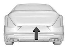
Press the touch pad on the rear of the trunk above the license plate when all doors are unlocked.
