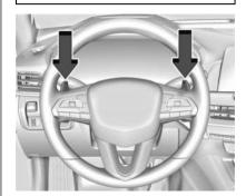
Vehicles with Manual Mode have controls on the back of the steering wheel to manually shift the automatic transmission. While using Manual Mode, the vehicle will have firmer, quicker shifting. You can use this for sport driving or when climbing or descending hills, to stay in gear longer, or to downshift for more power or engine braking.
