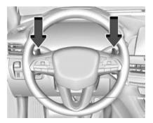
Vehicles with Manual Mode have controls on the back of the steering wheel to manually shift the automatic transmission.
