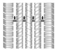
Treadwear indicators are one way to tell when it is time for new tires. Treadwear indicators appear when the tires have only 1.6 mm (1/16 in) or less of tread remaining. See *Tire Inspection* ⇔ 340 and *Tire Rotation* ⇔ 340.
