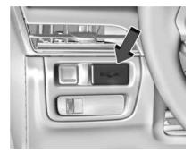
The PDR records video, audio, and vehicle data. This data is stored on a removable SD card located to the left of the steering wheel.
