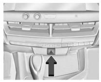
Press the **A** button to make the front and rear turn signal lights flash on and off. This warns others that you are having trouble. To turn the flashers off, release the button for at least one second and press again.
