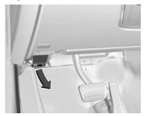
Pull the hood release lever with the symbol. It is on the lower left side of the instrument panel.
