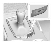
Driver Mode Control Switch for Manual Transmission
