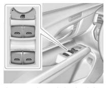
The power windows work when the vehicle is on, in accessory mode, or when Retained Accessory Power is active. See *Retained* Accessory Power (RAP) ⇒ 211.
