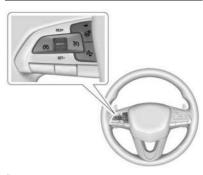
Press to turn the system on or off. The indicator turns white on the instrument cluster when ACC is turned on.
