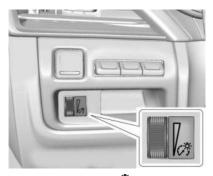
Rotate this thumbwheel  $\mathcal{E}^{\mathfrak{G}}$  up or down to adjust the brightness of all illuminated controls. The thumbwheel is on the instrument panel to the left of the steering wheel.
