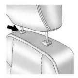
To lower the head restraint, press the button, located on the top of the seatback, and push the head restraint down. After releasing the button, ensure the head restraint locks in place and is unable to move up or down.
