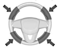
To begin steering manually, hold the steering wheel firmly with both hands using the highlighted regions. The Super Cruise light will display red and a message will display in the DIC. In addition, beeps will sound or the Safety Alert Seat will vibrate, if equipped. To view collision and detection settings, from the infotainment home screen, touch Settings > Vehicle > Collision/Detection Systems. When you begin steering manually, Super Cruise will disengage.
