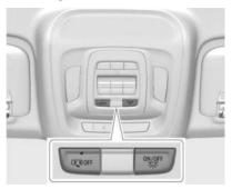
Dome lights provide overhead interior lighting for the front and rear seats. They may come on automatically as part of entry lighting and exit lighting, when and on the remote key is pressed, and can be turned on manually as needed.
