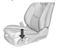
If equipped, the ignition must be on to use the massage feature.
