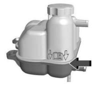
If coolant is visible but the coolant level is not at or above the indicated mark, add a 50/50 mixture of clean drinkable water and DFX-COOL coolant.
