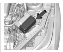
Lift the fuse block cover to access the fuses. The vehicle may not be equipped with all of the fuses and relays shown.
