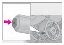
1 Press the Automatic High Beam switch.
