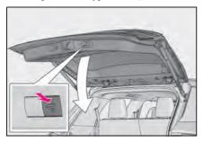
Close all of the doors except the back door, carrying an electronic key and press the switch on the lower part of the back door.
