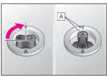
2 Turn the upper knob of each retaining hook (clip) to secure the floor mats in place.
