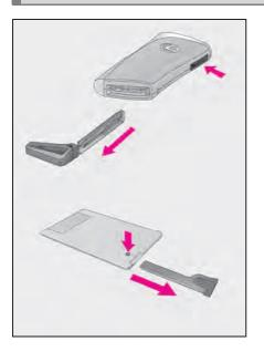
To take out the mechanical key, push the release button and take the key out.
