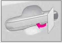
1 Insert a plastic card, etc. into the gap in the door handle to pry up the cover.
