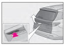
When the power back door is unlocked: Press the back door opener switch.
