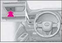
1 Press the switch to open the fuel filler door.
