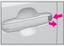
2 Remove the cover by pressing it on the rear.
