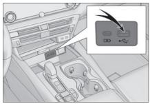
When connecting a USB flash drive, connect it directly to the USB port.
