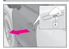
Press the door opener switch **A** of the door handle to open the door.
