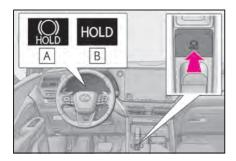
Turns the brake hold system on
