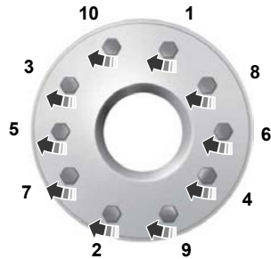
10-wheel nut torque sequence
