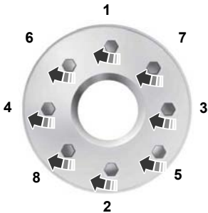
8-wheel nut torque sequence
