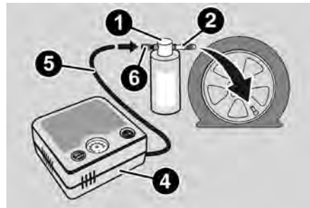
Attaching Filler Tube To Deflated Tire
