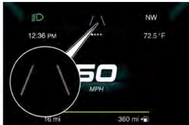
Lane Markings Not Detected
