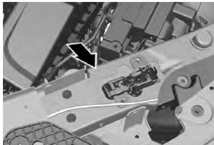
Protective Cover Location
