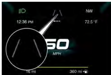
Lane Markings Not Detected
