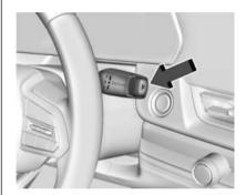
The shift pattern is displayed on the front of the shift lever. The selected gear position will illuminate red on the shift lever, while all others will be displayed in white. If the shift is not immediate, as in very cold conditions, the indicator on the shift switch may blink until it is fully engaged.
