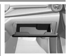
2. Squeeze both sides of the glove box bin inward to lower beyond the stops.
