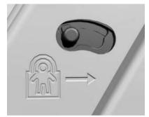
The safety lock is on the inside edge of the rear doors. To enable the safety lock:
