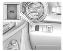
**AWD Mode:** AWD mode provides drive torque to all four wheels. Select AWD to improve traction and control on slippery road surfaces, such as gravel, sand, wet pavement, snow, and ice
