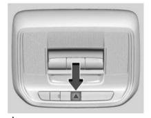
\(\to \): Press this button on the overhead console to make the front and rear turn signal lights flash on and off. This warns others that you are having trouble. Press again to turn the flashers off.
