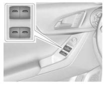
Power windows work when the vehicle is on, in accessory mode, or when Retained Accessory Power (RAP) is active. See *Retained Accessory Power (RAP)* ⇒ 168.
