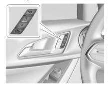
If equipped, the memory seat feature allows drivers to save their unique driving positions and a shared exit position.
