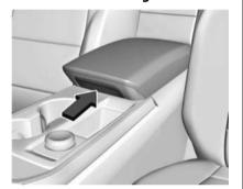
The center console has storage under the armrest. Press the button and lift to open.
