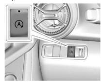
The automatic engine Stop/Start feature can be disabled and enabled by pressing (A). Stop/ Start is enabled each time you start the vehicle.
