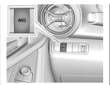
Press the All-Wheel Drive switch to activate the system. The indicator flashes briefly while the system engages and stays lit when the system is active. See *All-Wheel-Drive Light* ♀ 98.
