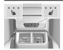
If equipped, the rear heated seat buttons are on the rear of the center console. To operate, the engine must be running.
