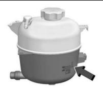
Check to see if coolant is visible in the coolant surge tank. If the coolant inside the coolant surge tank is boiling, do not do anything else until it cools down. If coolant is visible but the coolant level mark is not visible, add a 50/50 mixture of clean, drinkable water and DEX-COOL coolant at the coolant surge tank to the top rib on the middle of the tank, but be sure the cooling system is cool before this is done. See Engine Overheating \$\times 226\$.
