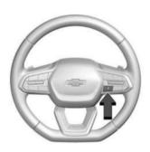
: If equipped with a heated steering wheel, press to turn on or off. A light near the button displays when the feature is turned on.
