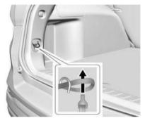
Route the loop end of the strap through one of the cargo tie-downs in the rear of the vehicle.
