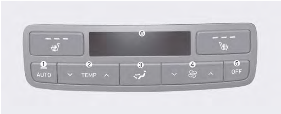
2nd row air conditioning control
