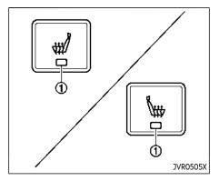
The front seats can be warmed by built-in heaters. The heating system of driver's seat and front passenger seat can be operated independently.
