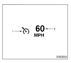
Conventional (fixed speed) cruise control mode display and indicators The display is located in the vehicle information display.
