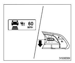
To set cruising speed, accelerate your vehicle to the desired speed, push the SET/ COAST (-) switch and release it. (The ICC system set indicator (green), vehicle ahead detection indicator, set distance indicator and set vehicle speed indicator come on.) Take your foot off the accelerator pedal. Your vehicle will maintain the set speed.
