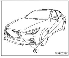
To display the multiple views, the Around View<sup>®</sup> Monitor system uses cameras ① located in the front grill, on the vehicle's outside mirrors and one just above the vehicle's license plate.
