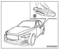
You can also unlock the corresponding door by touching the one touch unlock sensor (a) (driver's or front passenger's) within the range of operation, and can unlock the other doors using the door handle request switch
