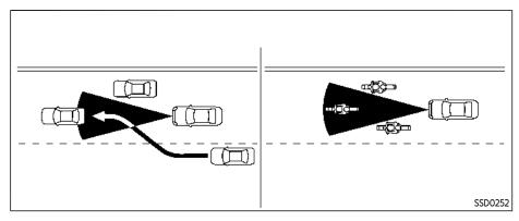
The detection zone of the radar sensor is limited. A vehicle ahead must be in the detection zone for the vehicle-to-vehicle distance detection mode to maintain the selected distance from the vehicle ahead.
