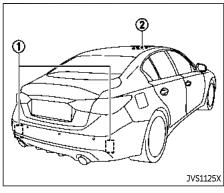
The BSI system uses radar sensors ① installed near the rear bumper to detect other vehicles in an adjacent lane. In addition to the radar sensors, the BSI system uses a camera ② installed behind the windshield to monitor the lane markers of your traveling lane.
