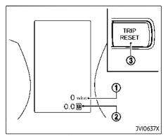
Odometer/twin trip odometer
