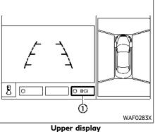
When the shift lever is placed in the R (Reverse) position, the indicator on the BCI system key (1) illuminates on the upper display.
