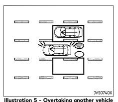
Illustration 5: If the driver activates the turn signal while another vehicle is in the detection zone, then the system chimes (twice) and the side indicator light flashes.
