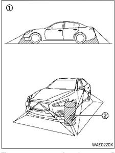
There are some areas where the system will not show objects and the system does not warn of moving objects. When in the front or rear view display, an object below the bumper or on the ground may not be viewed ①. When in the bird's-eye view, a tall object near the seam 2 of the camera viewing areas will not appear in the monitor.
