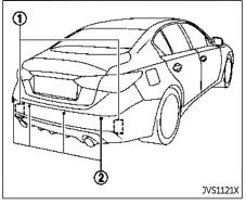
The BCI system uses radar sensors ① installed on both sides near the rear bumper to detect an approaching vehicle and sonar sensors 2 to detect objects in the rear.
