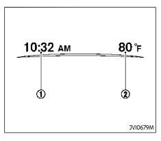
The outside temperature sensor is located in front of the radiator. The sensor may be affected by road or engine heat, wind directions and other driving conditions. The display may differ from the actual outside temperature or the temperature displayed on various signs, billboards or media information.
