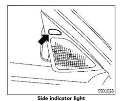
If the radar detects an approaching vehicle from the side, the system chimes (once), the side indicator light on the side the vehicle is approaching from flashes and a yellow rectangular frame ② appears on the upper display.
