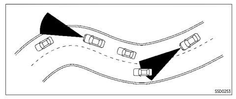
When driving on some roads, such as winding, hilly, curved, narrow roads, or roads which are under construction, the radar sensor may detect vehicles in a different lane, or may temporarily not detect a vehicle traveling ahead. This may cause the PFCW system to work inappropriately.
