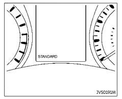
Multiple driving modes can be selected by using the INFINITI Drive Mode Selector (PERSONAL, SPORT+ (if so equipped), SPORT, STANDARD, ECO and SNOW).
