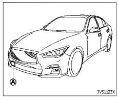
The FEB system uses a radar sensor (A) located behind the lower grille of the front bumper to measure the distance to the vehicle ahead in the same lane.
