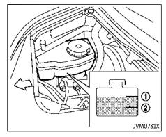
Check the fluid level in the reservoir. If the fluid is below the MIN line (2) or the brake warning light comes on, add Genuine NISSAN Super Heavy Duty Brake Fluid or equivalent **DOT 3** fluid up to the MAX line ①. If fluid must be added frequently, the system should be checked. It is recommended you visit an INFINITI retailer for this service.
