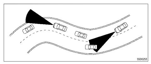
When driving on some roads, such as winding, hilly, curved, narrow roads, or roads which are under construction, the radar sensor may detect vehicles in a different lane, or may temporarily not detect a vehicle traveling ahead. This may cause the ICC system to decelerate or accelerate the vehicle.
