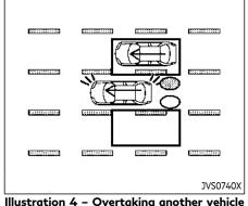
Illustration 4: If the driver activates the turn signal while another vehicle is in the detection zone, then the system chimes (twice) and the side indicator light flashes.
