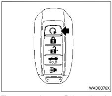
The remote engine start  $\Omega$  button is on the Intelligent Key if the vehicle has remote engine start function. This function allows the engine to start from outside the vehicle.
