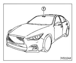
The LDW and LDP systems use a camera ① installed behind the windshield to monitor the lane markers of your traveling lane.
