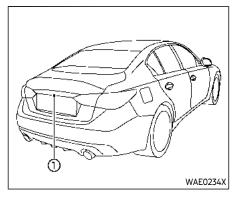
To display the rear view, the RearView Monitor system uses a camera ① located just above the vehicle's license plate.
