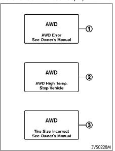
If the "AWD Error" warning @ appears, there may be a malfunction in the Intelligent AWD system. Reduce vehicle speed and have the system checked as soon as possible. It is recommended you visit an INFINITI retailer for this service.
