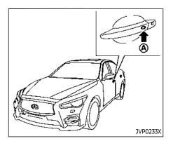
When you carry the Intelligent Key with you, you can lock all doors by pushing the door handle request switch (driver's or front passenger's) within the range of operation.
