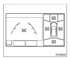
When the icon is displayed on the screen, the camera image may be receiving temporary electronic disturbances from surrounding devices. This will not hinder normal driving operation but the system should be inspected. It is recommended that you visit an INFINITI retailer for this service.
