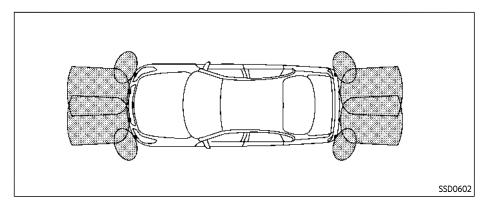
The sonar system sounds a tone to warn the driver of obstacles near the bumper. When the [Auto Show Sonar Image] key is turned on in the [Parking Sonar] settings, the sonar indicator will also appear on the upper display. (See "Sonar indicator" (P.5-137).)
