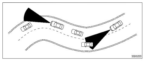
When driving on some roads, such as winding, hilly, curved, narrow roads, or roads which are under construction, the radar sensor may detect vehicles in a different lane, or may temporarily not detect a vehicle traveling ahead. This may cause the FEB system to work inappropriately.
