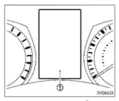
The vehicle information display ① is located between the tachometer and the speedometer, and it displays the warnings and information. The following items are also displayed if the vehicle is equipped with them:
