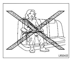
• Make sure the child's head will be properly supported by the booster seat or vehicle seat. The seatback must be at or above the center of the child's ears. For example, if a low back booster seat ① is chosen, the vehicle seatback must be at or above the center of the child's ears. If the seatback is lower than the center of the child's ears, a high back booster seat ② should be used.
