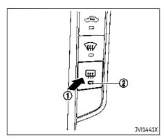
To defoq/defrost the rear window glass and outside mirrors, start the engine and push the switch (1) on. The indicator light (2) will come on. Push the switch again to turn the defroster off.
