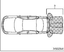
The radar sensors ① detect an approaching vehicle from up to approximately 49 ft (15 m) away. The sonar sensors ② detect stationary objects behind the vehicle up to approximately 4.9 ft (1.5 m). Refer to the illustration for approximate zone coverage areas ③.
