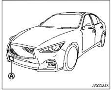
The PFCW system uses a radar sensor (A) located behind the lower grille of the front bumper to measure the distance to a second vehicle ahead in the same lane.
