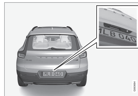
The rubberized button on the tailgate can only be used for unlocking.
