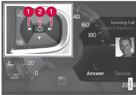
Examples of messages in the instrument panel 4 and the right-side steering wheel keypad.
