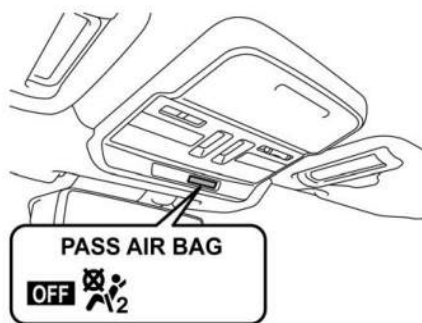
OFF Front passenger's frontal airbag OFF indicator light
