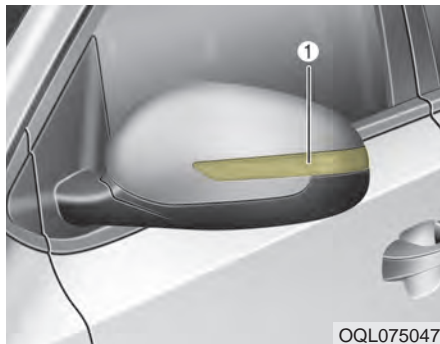
(1) Side repeater lamp (LED type)
