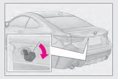
Turn the mechanical key clockwise to open.
