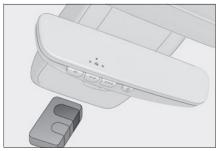
2 Point the remote control transmitter for the device at the rear view mirror, 1 to 3 in. (25 to 75 mm) from the HomeLink® buttons.
