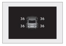
The tire pressure detected by the tire pressure warning system can be displayed on the multi-information display.
