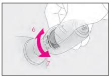
When AUTO mode is selected, the sensor sensitivity can be adjusted by turning the switch ring.
