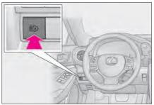
**1** Press the Automatic High Beam switch.
