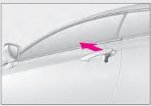
Insert the mechanical key while pulling on the driver's door handle.
