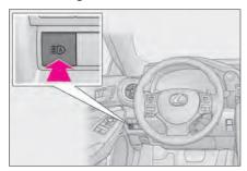
Press the Automatic High Beam switch.
