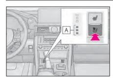
Each time the switch is pressed, the intensity of the seat ventilator changes and the level indicator lights (green) A light as follows:
