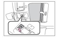
$<sup>^{\</sup>star 5}$ : Lightly press either end of the moon roof  $\iff$  switch to stop the moon roof while it is operating.
