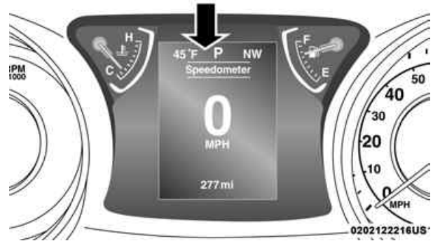
3.5 Inch Instrument Cluster Display Location
