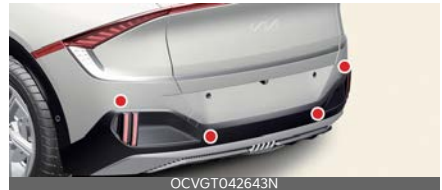
Rear ultrasonic sensors (Type C - GT)
