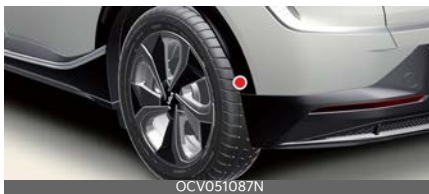
Rear side ultrasonic sensors
