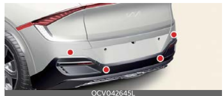
Rear ultrasonic sensors (Type C - GT)
