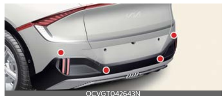
Rear ultrasonic sensors (Type C - GT)
