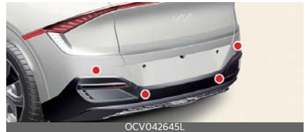
Rear ultrasonic sensors (Type C - GT)
