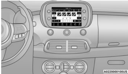
Automatic Climate Controls
