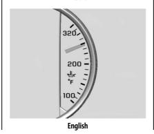
This gauge shows the engine oil temperature.
