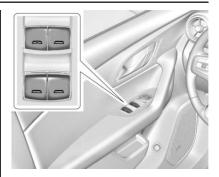
The power windows work when the ignition is on, in ACC/ACCESSORY, or when Retained Accessory Power (RAP) is active. See Retained Accessory Power (RAP) ⇒ 196.
