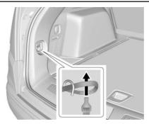
Place the loop end of the strap through the cargo tie-down. Place the hook end of the strap through the loop and pull it until the strap is fastened securely to the tie-down.
