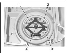
4. Turn the wing nut (4) counterclockwise to remove the jack (1), wheel wrench (2), and strap (3). Place the tool container near the tire being changed.
