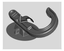
Insert one side of the load floor hook into the holder.
