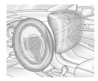
The driver frontal airbag is in the center of the steering wheel. The front outboard passenger frontal airbag is in the passenger side instrument panel.
