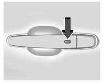
The remote key must be within 1 m (3 ft) of the liftgate or door being opened. Press the button on the door handle to unlock. See "Keyless Access Operation" in *Remote Key Operation*
