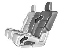
2. Pull the handle on the side of the seat cushion to unlock it.
