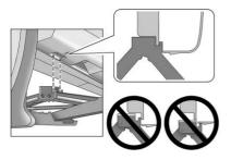
Turn the wheel wrench clockwise to raise the jack until the slot in the jack lift head fits into the metal flange located behind the cut out on the plastic molding.
