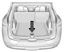
Lift the load floor to access the cargo management system.
