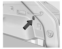
There is a shopping bag hook on each side of the rear cargo area. Press the hook to open. The maximum weight per hook is 5 kg (11 lb).
