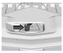
Go to the front of the vehicle and locate the secondary release lever under the front center of the hood. Push the secondary hood release lever to the right to release. After you have partially lifted the hood, the gas strut system will automatically lift the hood and hold it in the fully open position.
