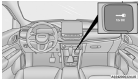
Front Power Outlet
