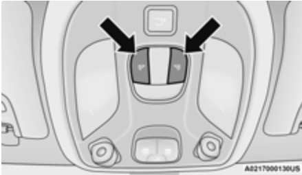
Overhead Light Switches
