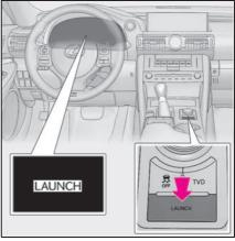
7 Firmly and fully depress the accelerator pedal. The control standby state will be entered and the engine speed will be automatically maintained between 1500-2000 rpm.
