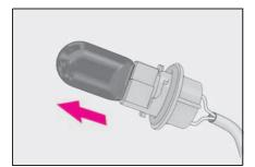
7 Install a new light bulb then install the bulb base to the light unit by inserting it and turning the bulb base clockwise.
