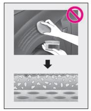
Do not apply a coating to the vehicle body, as it will form a film over the painted surfaces, filling the matte clear coat surface, making it more flat. As a result, it will become more glossy, possibly permanently losing its matte properties.
