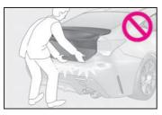
When closing the trunk lid, make sure to press it lightly on its outer surface. If the trunk handle is used to fully close the trunk lid, it may result in hands or arms being caught.
