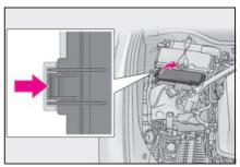
▶ Engine compartment: type B fuse box
