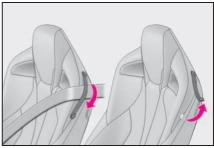
When fastening a front seat belt, ensure that it is passed through the seat belt guide. Passing the seat belt through the guide enables the seat belt to be easily extended.
