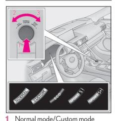
Normal mode and custom mode are selected by pressing the driving mode select switch. Each time the switch is pressed, the driving mode changes between normal mode and custom mode. When custom mode is selected, the "CUS-TOM" indicator will be illuminated.
