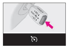
2 Accelerate or decelerate, with accelerator pedal operation, to the desired vehicle speed (at or above approximately 30 mph [50 km/h]) and push the lever down to set the speed.
