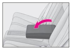
2 Separate the fastener and turn back the trunk door cover.
