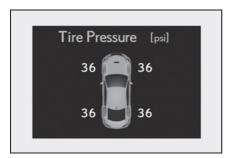
If the tire pressure drops below a predetermined level, the driver is warned by a screen display and a warning light. (→P.305)
