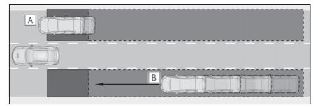
A Vehicles that are traveling in areas that are not visible using the outside rear
