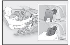
When the electronic key is detected, a buzzer sounds and the engine switch will turn to IGNITION ON mode.
