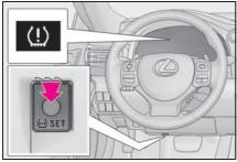
5 Wait for a few minutes with the engine switch in IGNITION ON mode and then turn the engine switch off.
