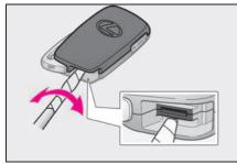
**3** Remove the depleted battery.
