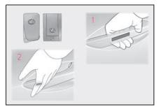
Grip the driver's door handle to unlock the door. Grip the passenger's door handle to unlock both side doors.\*
