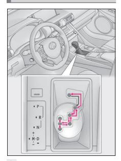
IGNITION ON mode, move the shift lever with the brake pedal depressed.
