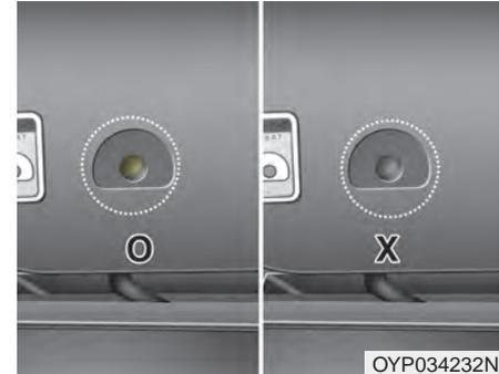
4. Make sure the green mark on the rear seat cushion frame is visible and the catches are locked in position by moving the seat forward and backward or lifting the front portion of the seat. If the green mark is invisible and the seat moves, it is not locked properly.
