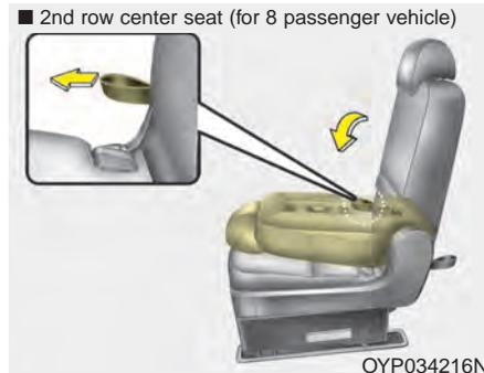
4. Pull on the seatback folding lever or strap, then fold the seat toward the front of the vehicle. When you return the seatback to its upright position, always be sure it has locked into position by pushing on the top of the seatback.
