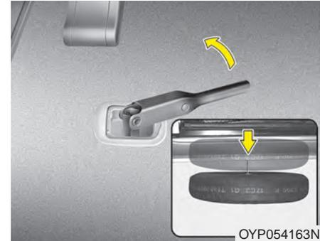
3. Use the wheel lug nut wrench to loosen the bolt enough to lower the spare tire.
