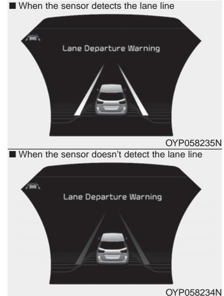
If the vehicle leaves the lane when the LDW operates and vehicle speed exceeds 40 mph (64 kph), the warning is issued as follows:
