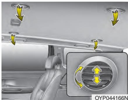
The vent can be adjusted by rotating the blade.
