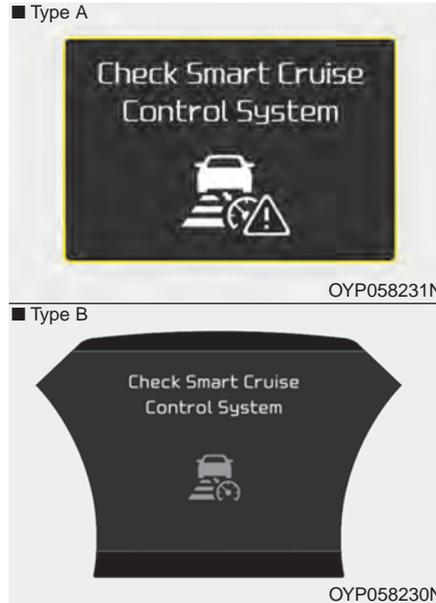
The message will appear when the vehicle to vehicle distance control system is not functioning normally. Take your vehicle to an authorized Kia dealer and have the system checked.
