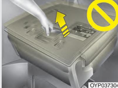
***Do not stow the 3rd row seat when the seat back is folded down. It may damage the 3rd seat mechanism.***
