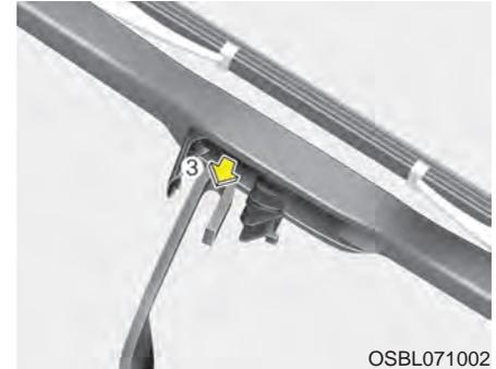
4. Push down the wiper arm (3) and install the new blade assembly in the reverse order of removal.
