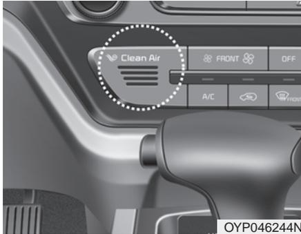
When the ignition switch is in the ON position, the clean air function turns on automatically.
