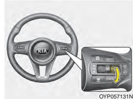
3. Move the lever down (to SET-), and release it at the desired speed. The set speed and vehicle to vehicle distance on the LCD screen will illuminate.
