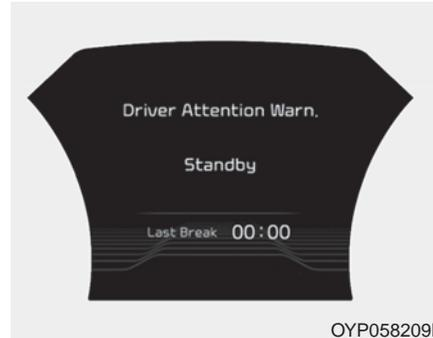
The Driver Attention Warning system enters the ready status and displays the 'Standby' screen in the following situations.
