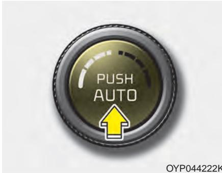
1. Press the AUTO button. The modes, fan speeds, air intake and air-conditioning will be controlled automatically by setting the temperature.
