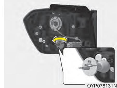
6. Remove the socket from the assembly by turning the socket counterclockwise until the tabs on the socket align with the slots on the assembly.
