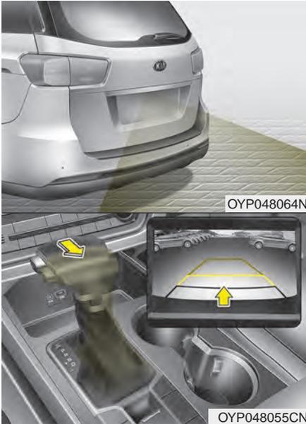
This system is a supplemental system that shows behind the vehicle through an AVN system screen while backing up.
