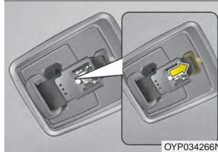
3. Insert the tongue plate into the holder (1) in seat belt and then insert the mini tongue into the hole on the belt assembly cover.
