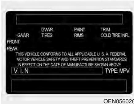
The certification label is located on the driver's door sill at the center pillar.
