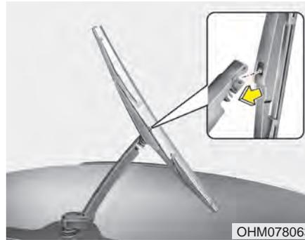
2. Install the new blade assembly by inserting the center part into the slot in the wiper arm until it clicks into place.
