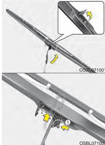
2. Turn the wiper blade clip. Then lift up the blade clip.
