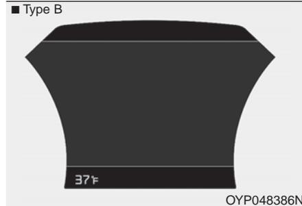
This gauge indicates the current outside air temperatures by 1°F (1°C).
