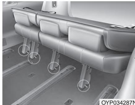
3. Make sure the catches are locked in position by moving the seat forward and backward or lifting the front portion of the seat. If the seat moves, it is not locked properly.
