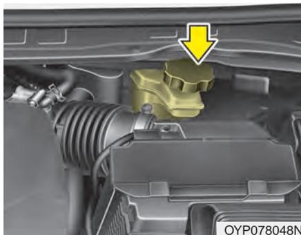
Check the fluid level in the reservoir periodically. The fluid level should be between MAX (Maximum) and MIN (Minimum) marks on the side of the reservoir.
