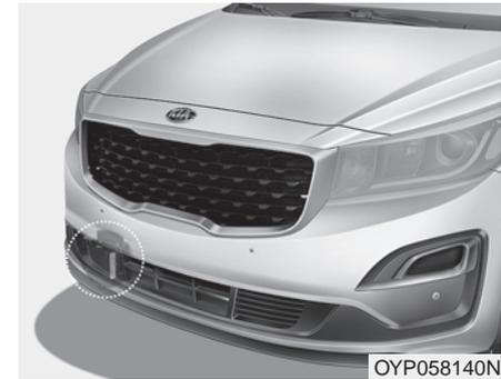
The sensor detects distance to the vehicle ahead.
