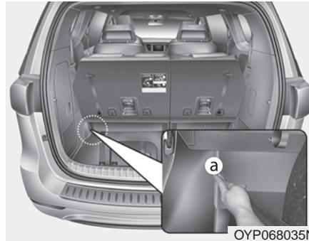
3. Connect the fixing belt to the striker (a) located at the bottom left/right side of the back of the third row seats.
