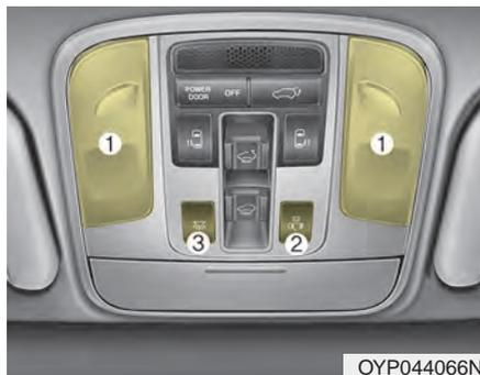
Press the lens (1) to turn the map lamp on or off
