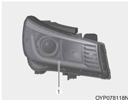
If the position lamp (LED) (1) does not operate, have the vehicle checked by an authorized Kia dealer.
