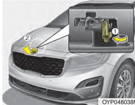
2. Go to the front of the vehicle, raise the hood slightly, pull up the secondary latch (1) inside of the hood center and lift the hood (2).
