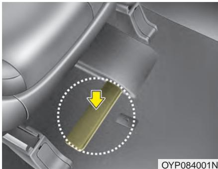
The vehicle identification number (VIN) is the number used in registering your vehicle and in all legal matters pertaining to its ownership, etc. The number is punched on the floor under the front passenger seat. To check the number, remove the cover.
