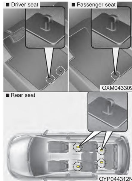
When using a floor mat on the front floor carpet, make sure it attaches to the floor mat anchor(s) in your vehicle. This keeps the floor mat from sliding forward.
