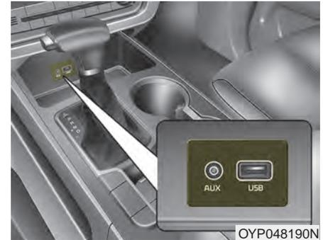
If your vehicle has an AUX and/or USB(universal serial bus) port, you can use an AUX port to connect audio devices and an USB and also an iPod®.
