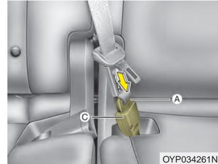
3. Insert the mini tongue (A) into the open end of the anchor connector (C) until an audible “click” is heard, indicating the latch is locked. Make sure the belt is not twisted.
