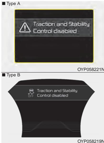
At this state, the engine control function and brake control function do not operate. It means the car stability control function does not operate any more.
