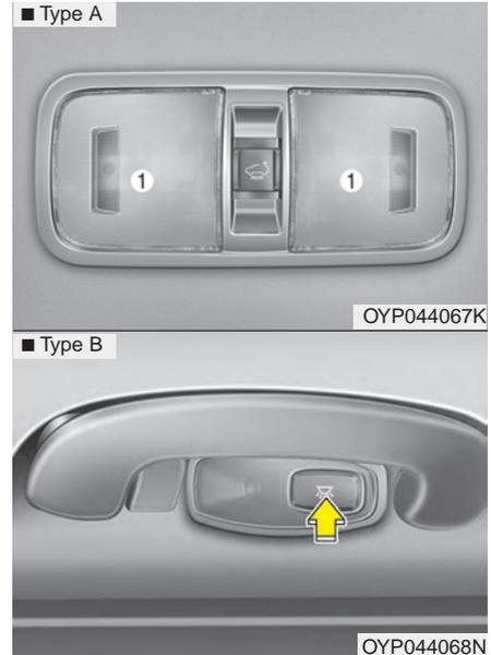
Press the button(1) or lens(1) to turn the light on or off.
