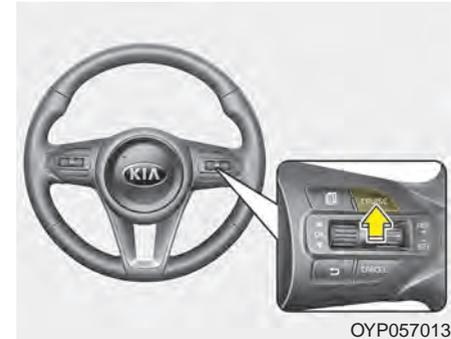
1. Press the CRUISE button on the steering wheel to turn the system on. The CRUISE indicator light in the instrument cluster will illuminate.
