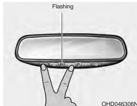
1. When programming the buttons for the first time, press and hold the left and center buttons (🏠, 🏠) simultaneously until the indicator light begins to flash after approximately 20 seconds. (This procedure erases the factory-set default codes. Do not perform this step when programming the additional HomeLink buttons.)
