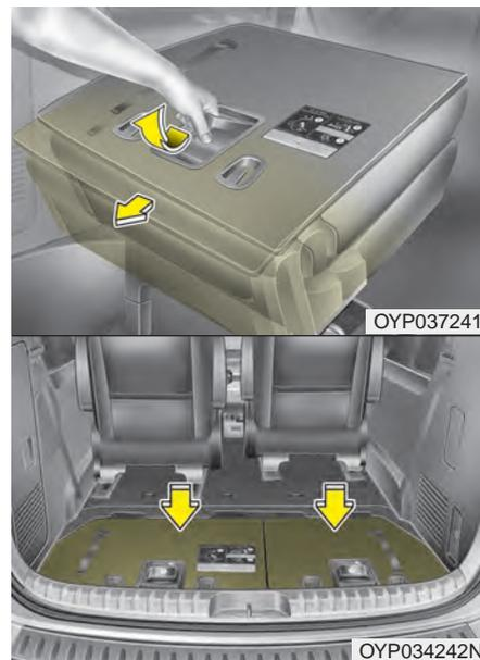
2. Pull up the seat by using the stowing lever.
