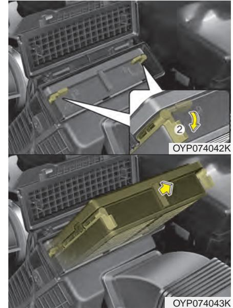
3. Wipe the inside of the air cleaner box. Be careful dust or dirt does not enter the air intake, or damage may result.
