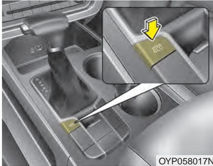
Active ECO helps improve fuel efficiency by controlling the engine and transaxle. But fuel-efficiency can be affected by the driver's driving habits and road conditions.
