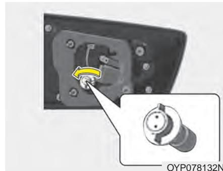
3. Remove the socket from the assembly by turning the socket counterclockwise until the tabs on the socket align with the slots in the assembly.
