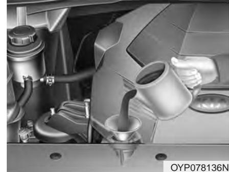
If it is near or at L, add enough oil to bring the level to F. **Do not overfill.**
