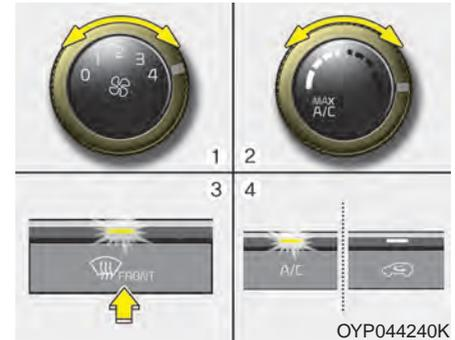
1. Set the fan speed to the desired position.
