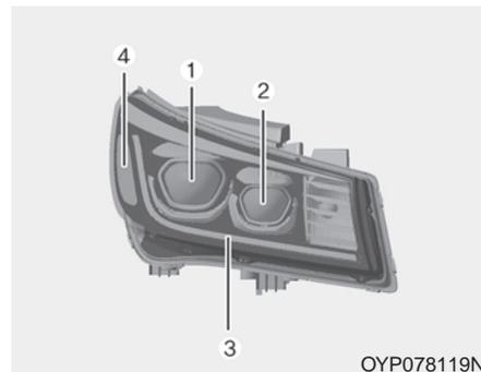
If the Low/High beam lamp(1), Low assist beam lamp(2), Position lamp(3) and Side marker (front)(4) does not operate, have the vehicle checked by an authorized Kia dealer.
