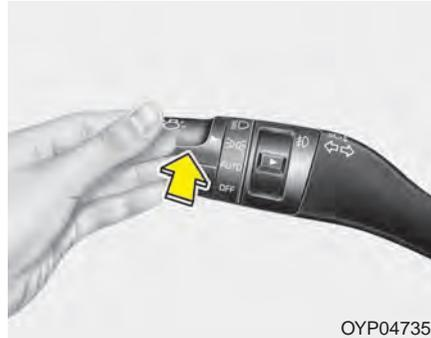
To turn on the high beam headlights, push the lever away from you. The lever will return to its original position.
