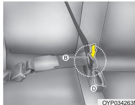
1. Press the release button on the buckle (D) and remove the tongue plate (B) from the buckle (D).
