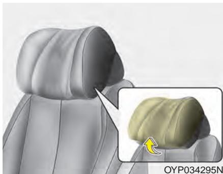
The headrest may be adjusted forward or backward by pulling the lower part of the headrest forward or backward to the desired detent in the direction of the arrow. Adjust the headrest so that it properly supports the head and neck.
