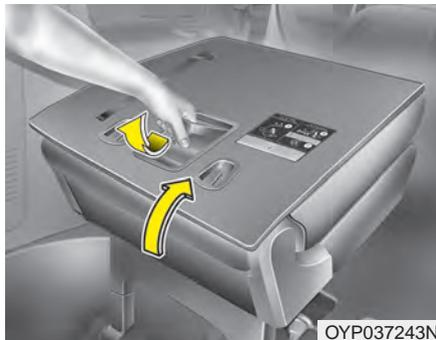
2. Release the lever and push the seat forward firmly until it clicks into place to insert the catches into the anchors.
