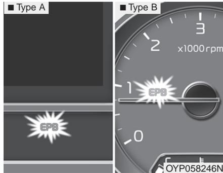
This warning light illuminates if the engine start/stop button is changed to the ON position and goes off in approximately 3 seconds if the system is operation normally.
