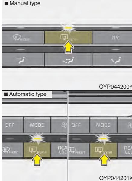
The defroster heats the window to remove frost, fog and thin ice from the rear window, while the engine is running.
