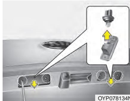
1. Using a screwdriver, the lamp assembly from lamp housing.
