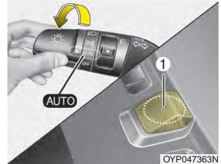
When the light switch is in the AUTO light position, the taillights and headlights will turn ON or OFF automatically depending on the amount of light outside the vehicle.
