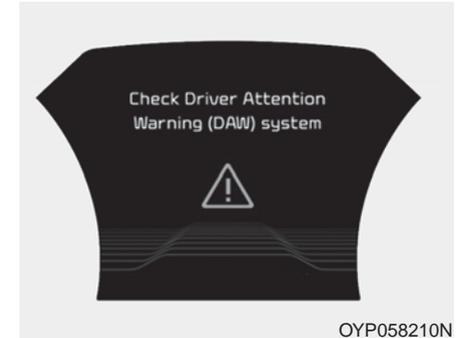
When the "Check Driver Attention Warning (DAW) system" warning message appears, the system is not working properly. In this case, have the vehicle inspected by an authorized Kia dealer.
