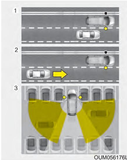
The Blind-Spot Collision Warning (BCW) system uses radar sensors in the rear bumper to monitor and warn the driver of an approaching vehicle in the driver's blind spot area.
