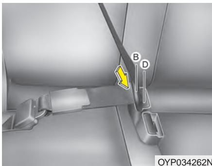
4. Pull the tongue plate (B) and insert the tongue plate (B) into the open end of the buckle (D) until an audible “click” is heard, indicating the latch is locked. Make sure the belt is not twisted.
