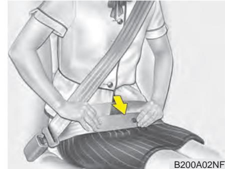
The seat belt automatically adjusts to the proper length only after the lap belt portion is adjusted manually so that it fits snugly around your hips. If you lean forward in a slow, easy motion, the belt will extend and let you move around. If there is a sudden stop or impact, however, the belt will lock into position. It will also lock if you try to lean forward too quickly.
