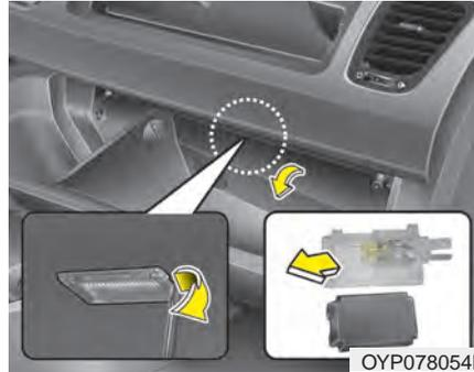
1. Using a flat-blade screwdriver, gently pry the lamp assembly from interior.
