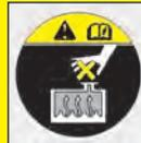
**Do not remove the radiator cap when the engine and radiator are hot. Scalding hot coolant and steam may blow out under pressure which may result in serious injury.**
