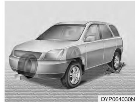
4. Remove the wheel lug nut wrench, jack and spare tire from the vehicle.
