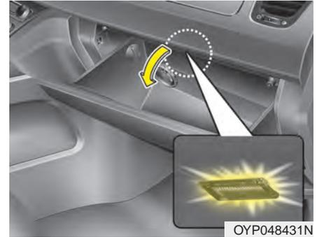
The glove box lamp comes on when the glove box is opened.
