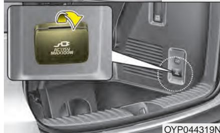
The AC inverter supplies 115V/100W electric power to operate electric accessories or equipments.
