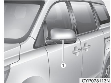
If the side repeater lamp (LED), does not operate, have the vehicle checked by an authorized Kia dealer. The LED lamps cannot be replaced as a single unit because it is an integrated unit. The LED lamps has to be replaced with the unit.
