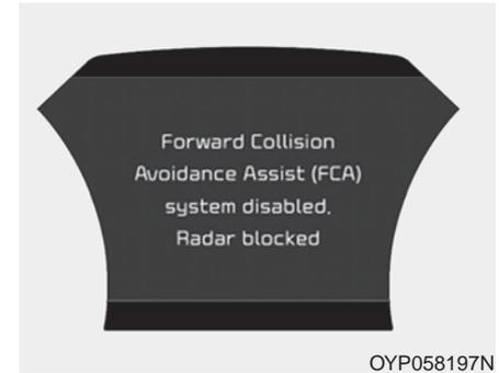
When the sensor cover or the sensor lens is smudged with the foreign substances, such as snow or rain, the FCA operation may temporarily stop. In this case, the warning message appears to warn the driver.
