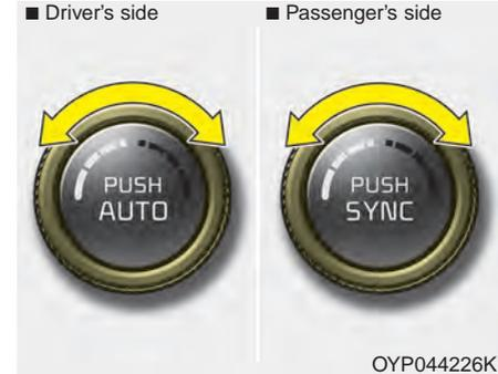
The temperature will increase to the maximum (HI) by turning the knob to the extreme right.
