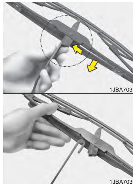
2. Compress the clip and slide the blade assembly downward.
