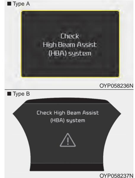
When the High Beam Assist is not working properly, the warning message will come on for a few second. After the message disappears, the master warning light (⚠) will illuminate.
