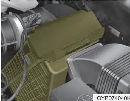
It must be replaced when necessary, and should not be washed. You can clean the filter when inspecting the air cleaner element.
