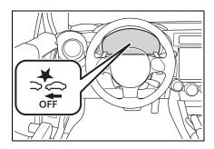
When the Pre-Collision Braking System OFF indicator is turned on, Pre-Collision Braking System (including the Pre-Collision Braking Assist function) and Pre-Collision Throttle Management do not operate.
