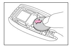
5 Align the protruding part with the slot and install the cover.
