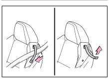
When fastening a front seat belt, ensure that it is passed through the seat belt guide. Passing the seat belt through the guide enables the seat belt to be easily extended.
