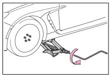
Securely tighten the wheel nuts two or three times in the order shown in the illustration using a wheel nut wrench.
