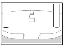
The area above the camera cannot be viewed. If there is an object that has a wide projection on its upper part such as a sign pole behind the vehicle, the projection cannot be seen on the screen.
