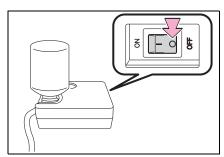
7 Connect the compressor power plug to the power outlet.
