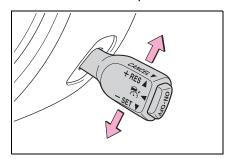
When Adaptive Cruise Control is activated, "READY" indicator turns off, the set vehicle speed is displayed, and changes from white to green.
