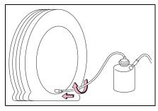
5 Turn the bottle upside down and tilt the bottle cap into the bottle holder of the air compressor.
