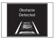
Vehicles in front in the same traffic lane are detected by the stereo camera within a distance of approximately 360 ft (110 m) in the forward direction. However the detection distance may be reduced depending on the traffic environment, driving conditions, and conditions of the vehicle in front.
