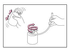
2 Connect the air compressor hose to the valve on the bottle.
