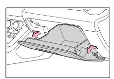
4 Lower the glove box slowly until surface (A) is horizontal with the floor, then pull it out. (Simply pulling with gentle
