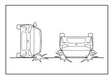
The angle of vehicle tip-up is marginal or the skidding vehicle's tires hit a curbstone laterally.
