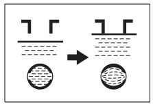
If the "UPPER LEVEL" line cannot be seen, check the fluid level by looking directly at the cell.
