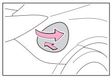
Turn the fuel tank cap slowly and remove it, then put it into the holder on the fuel filler door.
