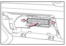
6 Remove the air conditioning filter and replace it with a new one.
