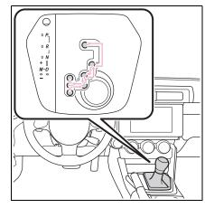
■ While the engine switch is in ON, move the shift lever with the brake pedal depressed.
