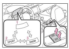
Press the sport mode switch or snow mode switch to change between normal mode and sport mode or snow mode respectively. To cancel sport mode or snow mode, press the same switch again.
