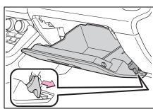
3 Push in each side of the glove box and pull the glove box toward you to disconnect the claws.
