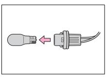
5 Install a new light bulb then install the bulb base to the light unit by inserting it and turning the bulb base clockwise.
