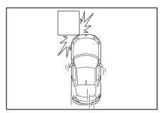
Examples of the types of accidents in which it is possible that the SRS side airbag and the SRS curtain shield airbag will deploy.
