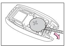
4 Install a new battery with the "+" terminal facing up, as shown in the illustration.
