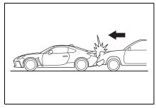
In an accident where the vehicle is impacted more than once, the driver's and/or front passenger's SRS frontal airbag(s) will deploy only once on the first impact of sufficient severity.
