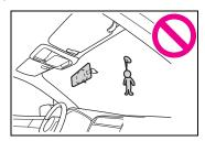
Do not attach accessories to the door trim or near either SRS side airbags and do not place objects near the SRS side airbags. In the event of SRS side airbag deployment, they could be propelled dangerously toward the vehicle's occupants and cause injuries.
