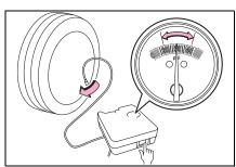
18If the air pressure is in red zone of the air gauge, the kit did not successfully seal the puncture. In this case, please stop driving and contact your Toyota dealer.
