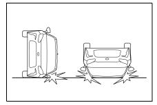
Examples of the types of accidents in which the SRS curtain shield airbag is unlikely to deploy.
