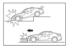
Examples of the types of accidents in which deployment of the driver's/driver's and front passenger's SRS frontal airbag(s) is unlikely to occur
