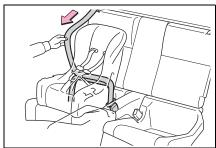
4 While pushing the child restraint system into the rear seat, allow the shoulder belt to retract until the child restraint system is securely in place.
