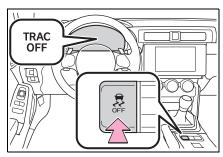
Within 5 seconds after the indicator lights turn off, release the switch. Then, press the switch again within 2 seconds of releasing it.
