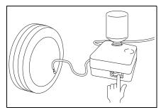
9 Adjust the air pressure to the appropriate level (green zone of the air gauge).
