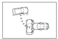
Examples of the types of accidents in which the driver's/driver's and front passenger's SRS frontal airbag(s) are not designed to deploy in most cases
