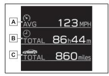
A Average vehicle speed Displays the average vehicle speed since display was reset.
