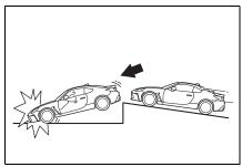
Examples of the types of accidents in which the SRS side airbag is unlikely to deploy.
