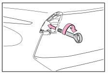
6 Tighten down the towing eyelet securely using a wheel nut wrench or hard metal bar.
