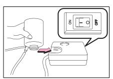
6 Make sure that the air compressor switch is off.
