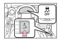
To turn the TRAC and VSC systems off, with the vehicle stationary, deactivate the TRAC system or select TRACK mode, and then press and
