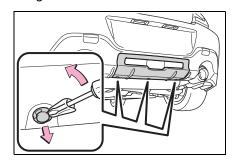
2 Pull the cover to disengage each claw and remove it.
