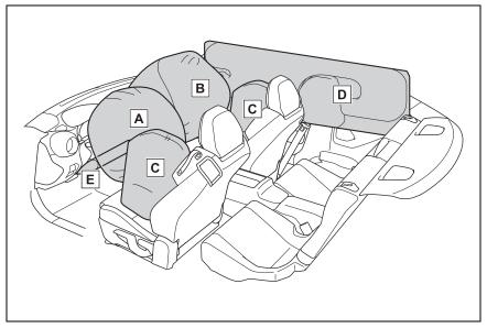
A Driver's SRS frontal airbag: in the center portion of the steering wheel
