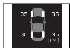
If the tire pressure drops below a predetermined level, the driver is warned by a screen display and a warning light. (→P.354)
