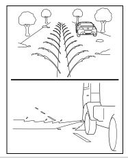
If there are installed accessories, etc. that are protruding beyond the edge of the front bumper, the vehicle's length will increase and the system may not be able to prevent a collision.
