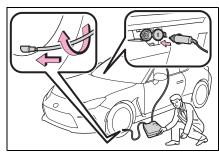
17Turn the compressor switch on and wait for several seconds, then turn it off. Check the tire inflation pressure.
