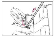
5 After installing the child restraint system, rock it back and forth to ensure that it is installed securely. (→P.70)
