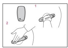
1 Grip the driver's door handle to unlock the door. Grip the passenger's door handle to unlock all the doors.\*
