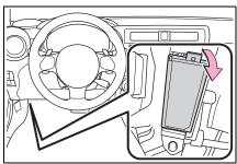
Remove the fuse with the pullout tool.
