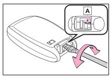
3 Remove the depleted battery.
