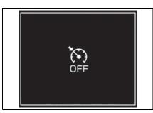
If EyeSight is malfunctioning, (yellow) is displayed on the meter display, and the Pre-Collision Braking System OFF indicator and Lane Departure Warning OFF indicator will also illuminate. If this occurs, stop the vehicle in a safe location and then turn off the engine and restart it. If the indica-
