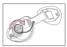
Close the fuel filler door, and press the center of the rear edge of the fuel filler door until you hear a click.
