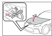
3 Hold the hood open by inserting the support rod into the slot. Hold the grip (A) for handling the hood prop.
