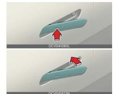
When all doors are closed, touch the touch sensor on the front outside door handle (the engraved part) while carrying the smart key with you, outside door handle will return and doors will be locked.
