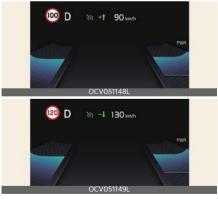
If the speed limit of the road changes during the operation of Manual Speed Limit Assist or Smart Cruise Control, an arrow in the direction of up or down is displayed to inform the driver that the set speed needs to be changed. At this
