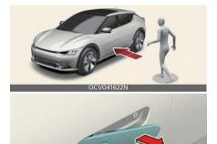
If you approach (within 30 cm (1 ft.)) the driver or front passenger's door handle possessing the smart key, the outside door handles slide out and the doors are unlocked. In this case, Hazard Warning Flasher blinks twice and chime also sounds twice.
