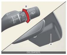
The rain sensor (A) located on the upper end of the windshield glass senses the amount of rainfall and controls the wiping cycle for the proper interval. The more it rains, the faster the wiper operates. When the rain stops, the wiper stops.
