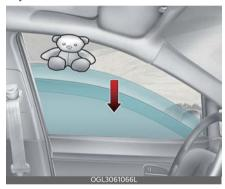
If the window detects the resistance while the power window switch is pulled up continuously, the window will stop upward movement then lower approximately 2.5 cm (1 inch).
