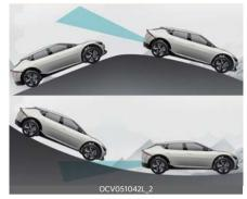
Blind-Spot Collision-Avoidance Assist may not operate properly when driving on a sloped road. Blind-Spot Collision-Avoidance Assist may not detect the vehicle in the next lane or may incorrectly detect the ground or structure.
