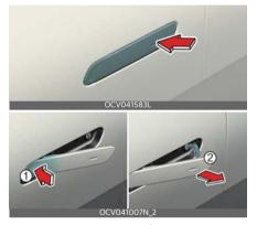
Push the button on the front outside door handle (the engraved part) while carrying the Smart Key with you, all doors will unlock.
