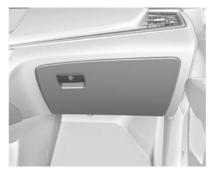
Lift the handle to open the glove box. Close until it latches. Use the vehicle key to lock or unlock.
