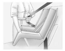
4. Pull the shoulder belt all the way out of the retractor to set the lock. When the retractor lock is set, the belt can be tightened but not pulled out of the retractor.
