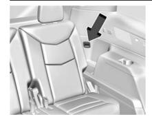
Insert the SD card into the card reader in the trim panel of the left-hand rear seat. Disable the system from the playback screen before removing the SD card from the reader. Do not remove the card while recording is enabled. This could corrupt the video file and/or the SD card.
