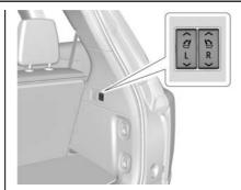
To return the seatback to the seating position from the cargo area, press and hold the seatback folding switch on the passenger side of the rear cargo area.
