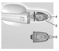
2. Insert the two tabs (6) at the back of the cap between the seal (5) and the metal base (4).
