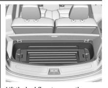
Lift the load floor to access the cargo management system storage area.
