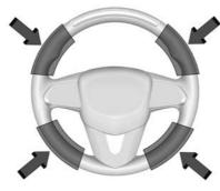
Any time the steering wheel light bar flashes red, resume manual steering immediately. The instrument cluster light , will also turn red and a message will display in the Driver Information Center (DIC). In addition, beeps will sound, or the Safety Alert Seat will vibrate. See "Collision/ Detection Systems" under *Vehicle Personalization* \$\to\$ 130. After you begin steering manually, then Super Cruise will disengage.
