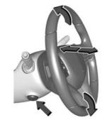
Power Tilt and Telescoping Steering Wheel
