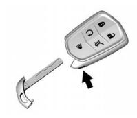
Press the button on the side of the RKE transmitter near the bottom and pull the key out. Never pull the key out without pressing the button.
