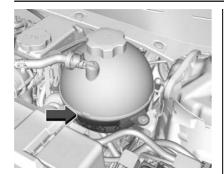
Check to see if coolant is visible in the coolant surge tank. If the coolant inside the coolant surge tank is boiling, do not do anything else until it cools down. If coolant is visible but the coolant level mark is not at or above the indicated mark, add a 50/50 mixture of clean, drinkable water and DEX-COOL coolant. Be sure the cooling system is cool before this is done. See *Engine Overheating* \$334.
