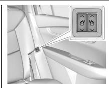
To fold the third row seatback from the second row seating area, press and hold the seatback folding switch on the right or left side of the second row seating area.
