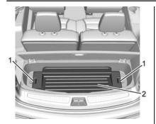
Remove the cargo management system tray (2) by pulling on the handles (1).
