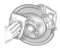
Remove any rust or dirt from the wheel bolts, mounting surfaces, and spare wheel. 11. Place the spare tire on the wheel-mounting surface.
