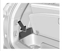
The rear compartment fuse block is in the cargo area, on the driver side of the vehicle behind the lower trim panel. To access the fuses in the Rear Electrical Center, remove the center cargo bin, then small side bin. See *Rear Storage* ⇔ *93.* See your dealer if additional assistance is needed.
