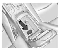
3. Place the new transmitter into the transmitter pocket. The transmitter pocket is inside the center console storage area between the driver and front passenger seats. The storage area will need to be opened and the storage tray lifted up to access the transmitter pocket.
