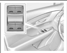
The power windows work when the ignition is on, in ACC/ACCESSORY, or when Retained Accessory Power (RAP) is active. See *Retained Accessory Power (RAP)* ⇒ 236.
