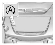
The automatic engine Stop/Start feature can be disabled and enabled by touching the  $\bigcirc$  symbol. Auto Stop is enabled each time you start the vehicle.
