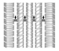
Treadwear indicators are one way to tell when it is time for new tires. Treadwear indicators appear when the tires have only 1.6 mm (1/16 in) or less of tread remaining. See *Tire Inspection*  $\Rightarrow$  364 and *Tire Rotation*  $\Rightarrow$  365 for additional information.
