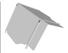
Open both crossbars until the center hinge locks. Keep fingers clear of the crossbar hinges to avoid being pinched.
