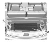
3. Remove the cargo management system tray (2) by pulling on the handles (1). See *Cargo Management System* \$ 97.
