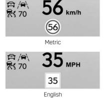
Speed View: This displays digital speed in English or metric units, speed limit, and indicators such as vehicle ahead, Lane Departure Warning/Lane Keep Assist, and Adaptive Cruise Control and set speed. Some information only appears on vehicles that have these features, and when they are active.
