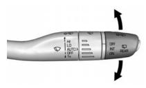
The rear window wiper/washer controls are on the end of the windshield wiper lever.
