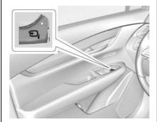
If equipped, press  $\Box_i$  to power fold the mirrors. Press  $\Box_i$  again to unfold.
