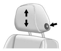
To raise or lower the head restraint, press the button located on the side of the head restraint, and pull up or push the head restraint down, and release the button. Pull and push on the head restraint after the button is released to make sure that it is locked in place.
