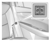
To return the seatback to the seating position from the second row seating area, press and hold the seatback folding switch on the right or left side of the second row seating area.
