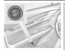
The power liftgate switch is on the driver door. The vehicle must be in P (Park).
