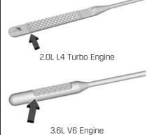
If the oil is below the cross-hatched area at the tip of the dipstick and the engine has been off for at least 15 minutes, add 1 L (1 qt) of the recommended oil and then recheck the level. See "Selecting the Right Engine Oil" later in this section for an explanation of what kind of oil to use. For engine oil crankcase capacity, see Capacities and Specifications
