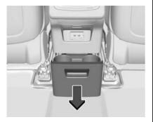
If equipped with cupholders in the back center console, pull on the handle to access.
