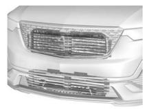
The vehicle may have a shutter system designed to help improve fuel economy. Keep the shutter system clear of debris, snow and ice. If the check engine light is activated, please check to see if the shutter system is clear of debris, snow or ice.
