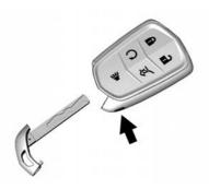
To remove the key, press the button on the side of the transmitter, near the bottom, and pull the key out. Never pull the key out without pressing the button.
