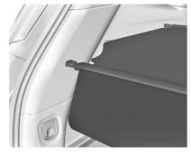
8. Insert the two rearward ends into the remaining slots on each side.
