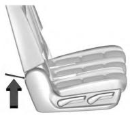
Pull the strap on the bottom rear of the second row seat to release the seatback. The seatback will fold forward.
