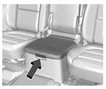
If equipped with front center seat storage, unlock with the mechanical key inside the remote key. See  $Keys \Leftrightarrow 7$ .
