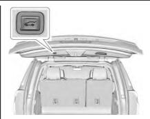
• Press on the bottom edge of the liftgate next to the latch to close.
