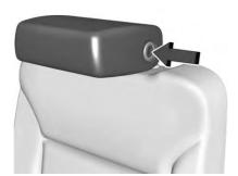
The head restraint will fold forward automatically.
