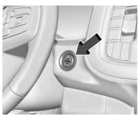
Vehicles equipped with Keyless Access have pushbutton starting.
