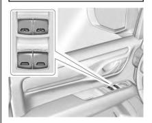
The power windows work when the ignition is on, in ACC/ACCESSORY, or when Retained Accessory Power (RAP) is active. See Retained Accessory Power (RAP) ⇒ 229.
