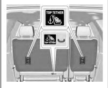
The top tether anchors are on the rear of the seatback for the outboard seating positions and the rear of the seat cushion for the center seating position in the second row. Be sure to use an anchor located directly behind the seating position where the child restraint will be placed.
