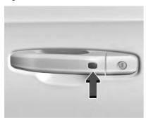
The remote key must be within 1 m (3 ft) of the trunk or door being opened or locked. Press the button on the door handle to open. See "Keyless Access Operation" in Remote Keyless Entry (RKE) System Operation
