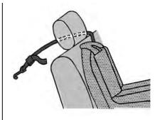
If the position you are using has a fixed headrest or head restraint and you are using a single tether, route the tether around the inboard side of the headrest or head restraint.
