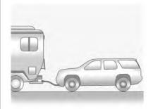
Only dinghy tow four-wheel-drive vehicles with a two speed transfer case that has an N (Neutral) and a  $4\rlap{\downarrow}$  setting.
