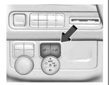
The brightness of the instrument cluster display, infotainment display and controls, steering wheel controls, and all other illuminated controls, as well as feature status indicators can be adjusted.
