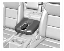
To move the armrest forward, push forward on the center of the armrest with the palm of your hand.
