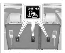
For the third row seat, the top tether anchors are on the back of the seatback. Be sure to use an anchor located directly behind the seating position where the child restraint will be placed.
