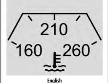
This gauge measures the temperature of the vehicle's engine coolant.
