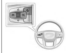
**RES+**: Press briefly to resume the previous set speed or to increase vehicle speed if ACC is already activated. To increase speed by about 1 km/h (1 mph), press RES+ briefly. To increase speed to the next 5 km/h (5 mph) mark on the speedometer, hold RES+.
