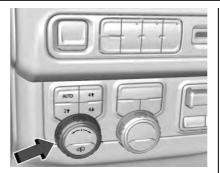
To activate each mode, turn the Mode knob on the instrument panel to the left of the steering wheel.
