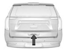
To open the liftgate, press on the power door lock switch or press on the remote key twice to unlock all doors. Press the touch pad (1) on the underside of the liftgate handle and lift up.
