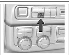
Press are to enable or disable HDC. Vehicle speed must be below 60 km/h (37 mph).
