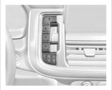
The shift switches are on the center stack. The selected gear position will illuminate red on the shift switch, while all others will be displayed in white. If the shift is not immediate, as in very cold conditions, the indicator on the shift switch may blink until it is fully engaged.
