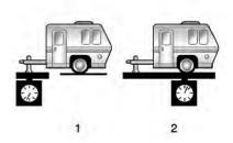
The trailer tongue weight (1) should be 10–15% of the total loaded trailer weight (2). Some specific trailer types, such as boat trailers, fall outside of this range. Always refer to the trailer owner's manual for the recommended trailer tongue weight for each trailer. Never exceed the maximum loads for the vehicle, hitch, and trailer.
