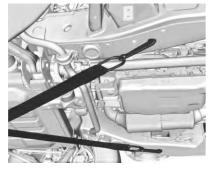
The vehicle is equipped with specific attachment points to be used to pull the vehicle onto a flathed car carrier from a flat road surface. Do not use these attachment points to pull the vehicle from snow, mud or sand.
