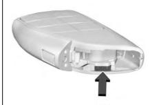
With the mechanical key removed, insert a flat, thin object in the center of the remote key to separate and remove the back cover.
