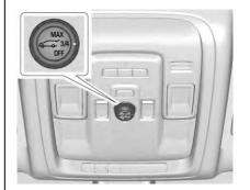
If equipped, the power liftgate switch is on the overhead console. The vehicle must be in P (Park).
