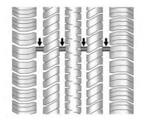
Treadwear indicators are one way to tell when it is time for new tires. Treadwear indicators appear when the tires have only 1.6 mm (1/16 in) or less of tread remaining. See *Tire Inspection* ⇒ 350 and *Tire Rotation* ⇒ 350 for additional information.
