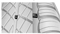
Wear indicators are distributed around the tire circumference. These wear indicators have the legally required minimum height of 0.063 in/1.6 mm
