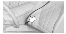
When the safety belt is fastened, the driver's and front passenger's belt straps are automatically tightened once after driving away.
