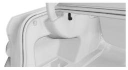
A multifunction hook is located on the left and right side in the cargo area.
