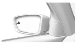
The light in the exterior mirror flashes if vehicles are detected by the rear sensors and your own vehicle is moving in reverse.
