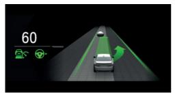
Example: the indicator/warning lights for the Active Cruise Control with Stop & Go function ACC and the Lane Change Assistant indicate a lane change to the next lane. At the same time, the lane change to the next lane is shown with animation in the Assisted Driving View.
