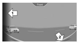
The respective boundary area, arrow 1, in the camera view flashes red, if vehicles are detected by the sensors.
