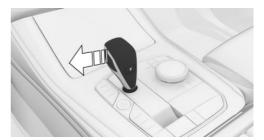
Press the selector lever to the left from selector lever position D.
