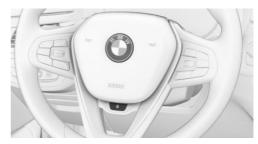
Button for steering wheel heating
