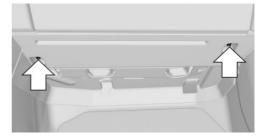
Loosen fasteners, arrows, and open cover.
