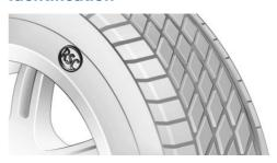
The tires are marked on the tire sidewall with Run-flat System Component RSC.
