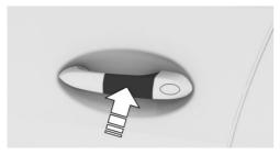
Hold activated Key Card directly and centered on the external door handle of the driver's door. If the Key Card is not detected, slightly change the position of the Key Card and repeat the procedure.
