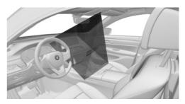
The camera in the headliner detects gestures that are carried out in the area of the center console at the height of the Control Display.
