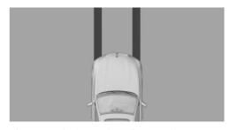
The car wash view assists when entering a car wash by displaying the floor and the vehicle's own track.
