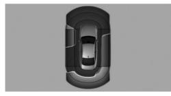
To protect the sides of the vehicle, obstacle markings are displayed on the sides of the vehicle.
