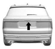
To open the liftgate, press the touch pad in the liftgate handle and lift up.
