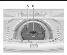
If the vehicle is equipped with a subwoofer (5), remove the center wing nut (6), then remove the subwoofer and set it aside. Do not disconnect the wiring harness.
