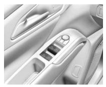
The power windows work when the vehicle is on, in accessory mode, or when Retained Accessory Power (RAP) is active. See *Retained Accessory Power* (RAP)  $\Rightarrow$  184.
