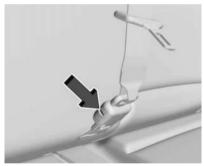
4. Disconnect the center seat belt mini-latch, using a key in the slot on the mini-buckle, and let the belt retract into the headliner.
