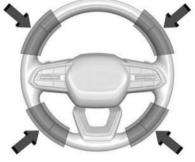
To begin steering manually, hold the steering wheel firmly with both hands using the highlighted regions shown.
