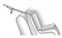
If the position you are using does not have a head restraint and you are using a single tether, route the tether over the seatback.
