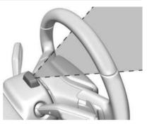
Sunglasses, hats, or other types of clothing that change the shape of the head may interfere with camera performance. To improve camera performance, raise or lower the steering wheel, or change the seat position.
