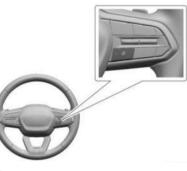
If equipped, press to turn the heated steering wheel on or off. A light next to the button displays when the feature is turned on.
