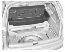
4. The load floor and storage bin can be placed on the lowered third row seats while accessing the spare tire.
