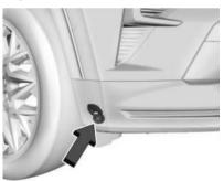
If equipped, the engine heater can provide easier starting and better fuel economy during engine warm-up in cold weather conditions at or below -18 °C (0 °F). Vehicles with an engine heater should be plugged in at least four hours before starting. An internal thermostat in the plug-end of the cord may exist, which will prevent engine heater operation at temperatures above –18 °C (0 °F).
