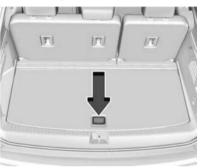
There is storage under the floor of the rear cargo area. Lift the handle to access the cargo management system.
