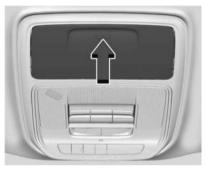
Sunglasses storage is on the overhead console. Press the cover and release to access.
