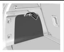
1. If equipped, there may be an outer panel that needs to be removed to get to the inner panel. Press the clip and pull the panel towards you to remove the panel.
