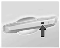
The remote key must be within 1 m (3 ft) of the liftgate or door being opened. Press the button on the door handle to open. See *Remote Key Operation*  $\Leftrightarrow$  7.
