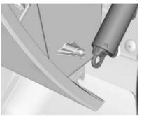
3. Disconnect the glove box door damper from the glove box door assembly by squeezing the pivot to release the damper ring.
