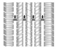
Treadwear indicators are one way to tell when it is time for new tires. Treadwear indicators appear when the tires have only 1.6 mm (1/16 in) or less of tread remaining. See *Tire Inspection*  $\Rightarrow$  301 and *Tire Rotation*  $\Rightarrow$  301.
