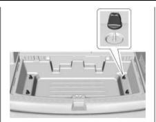
2. Remove the four wing nuts.
