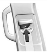
Press and hold the release button while raising or lowering the height adjuster to the desired position.
