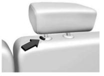
The height of the head restraint can be adjusted. Pull the head restraint up to raise it. Try to move the head restraint to make sure that it is locked in place. To lower the head restraint, press the button, located on the top of the seatback, and push the head restraint down.
