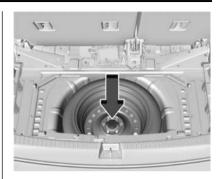
9. If the vehicle is not equipped with a subwoofer, remove the center wing nut, then remove the spare tire and place it next to the tire being changed.
