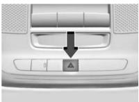
A: Press this button on the overhead console to make the front and rear turn signal lamps flash on and off. This warns others that you are having trouble. Press again to turn the flashers off.
