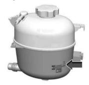
Check to see if coolant is visible in the coolant surge tank. If the coolant inside the coolant surge tank is boiling, do not do anything else until it cools down. If coolant is visible but the coolant level mark is not visible, add a 50/50 mixture of clean, drinkable water and DEX-COOL coolant at the coolant surge tank to the top rib on the middle of the tank, but be sure the cooling system is cool before this is done. See Engine Overheating  $\Rightarrow$  273.
