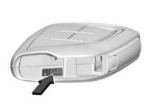
2. Separate the two halves of the remote key by using the blade of the mechanical key inserted into the bottom center of the remote key. Do not use the key slot.
