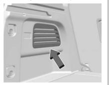
2. The inner panel is removed by prying along the top edge of the trim panel. Remove the trim panel to access the fuse block, or see your dealer.
