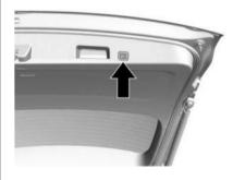
Press I on the bottom of the liftgate to close.
