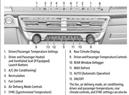
controlled by touching CLIMATE on the infotainment home screen. A selection can then be made on the climate control page displayed.
