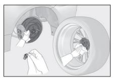
2 Align a wheel bolt hole on the spare tire with the guide pin and install the spare tire
