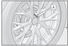
6 Remove the remaining wheel bolts and the tire.
