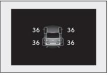
If the tire pressure drops below a predetermined level, the driver is warned by a screen display and a warning light. (→P.315)
