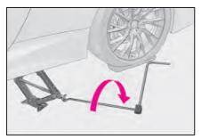
5 Remove the uppermost wheel bolt and install the guide pin by hand.
