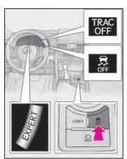
■ When the "TRAC OFF" indicator light comes on even if the switch has not been pressed
