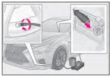
**21** Turn the compressor switch on for a few seconds and then turn it off and check the tire inflation pressure.
