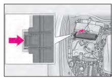
▶ Engine compartment: type B fuse hox
