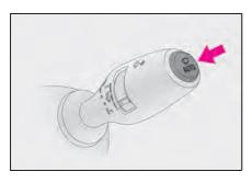
Operation of the intermittent windshield wipers with interval adjuster
