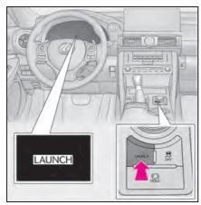
7 Firmly and fully depress the accelerator pedal.
