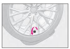
**6** Extend the hose and remove the air release cap.
