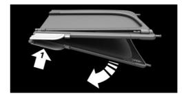
2. Open the rear side window, if necessary. Insert wind deflector from one side of the vehicle with the pins in the corresponding fixing points on the opposite side of the vehicle.
