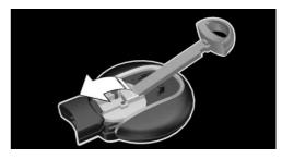
Push battery in the direction of the arrow using a pointed object and lift it out.
