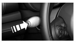
Reset the current driving time: press button on the turn signal lever for approx. 2 seconds with the driving times displayed.
