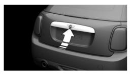
Press the button on the exterior of the trunk lid.
