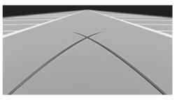
Turning radius lines can be superimposed on the image of the rearview camera.
