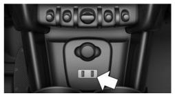
Depending on the vehicle equipment, one or two USB interfaces are located in the front of the center console.
