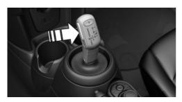
With the driver's safety belt fastened, briefly push the selector lever in the desired direction, past a resistance point, if needed. The selector lever automatically returns to the center position when released.
