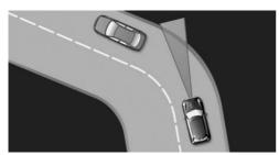
If the desired speed is too high for a curve, the speed is reduced slightly, although curves cannot be anticipated in advance. Therefore, drive into a curve at an appropriate speed.
