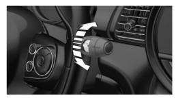
Turn the thumbwheel on the wiper lever.
