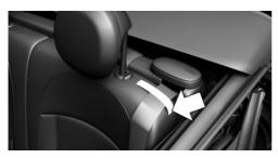
When fastening the safety belts on the rear seats, make sure that the belt loop is closed.
