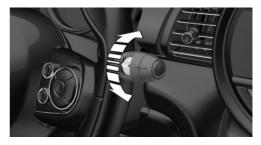
Turn the thumbwheel on the wiper lever.
