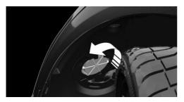
Turn the bulb socket counterclockwise and remove it from the bulb housing.
