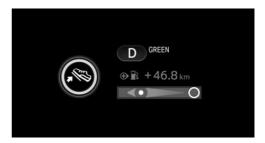
The GREEN tip indicates that your driving style can be modified to be more efficient, for example by backing off the accelerator.
