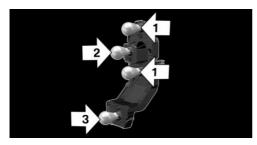
6. Proceed in the reverse order to insert the new bulb and attach the bulb holder. Make sure that the bulb holder engages in all fasteners.
