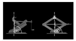
6. Make sure that the vehicle jack foot stands vertically and perpendicularly beneath the jacking point after extending the vehicle jack.
