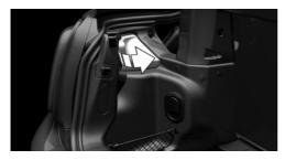
Turn the bulb holder for the reversing light, arrow, counterclockwise and remove it.
