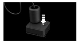
Let the compressor run for max. 10 minutes to fill the tire with sealant and achieve a tire inflation pressure of approx. 2.5 bar. While the tire is being filled with sealant,
