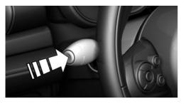
Press the button on the turn signal lever. Information is displayed in the Info Display of the instrument cluster.
