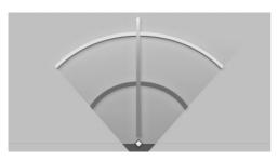
Two static circle segments show the distance between the trailer and the trailer hitch.
