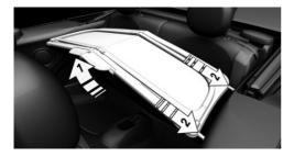
5. Press the wind deflector downward in the middle, until the handle engages, arrows 1.
