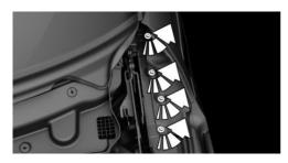
Turn the bulb socket counterclockwise and remove.
