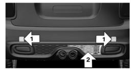
The fixing points, arrow 1, and the socket, arrow 2, are located below the covers in the bumper.
