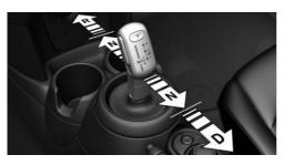
The selector lever positions P, R, N, and D are selected by tapping the selector lever forward or back. The selector lever automatically returns to the center position when released.
