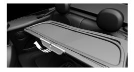
4. Press the wind deflector inwardly and up, arrow 1, to the extent that the wind deflector can be positioned in front of the fixing points on the installation side. Release the handle.
