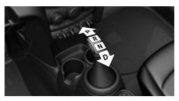
The selector lever positions P, R, N, and D are selected by moving the selector lever into the respective selector lever position. The selector lever engages in the selector lever positions.
