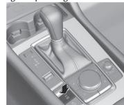
When the parking brake is released, the EPB indicator light (E) in the instrument cluster and the EPB switch indicator light turn off.
