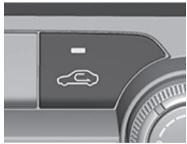
The mode is switched between recirculate mode and fresh air mode each time the switch is pressed.
