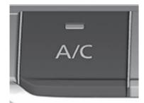
The cooling/dehumidifying function switches between on and off each time the switch is pressed. The indicator light turns on while the function is operating.
