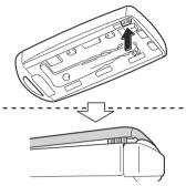
Insert a tape-wrapped flathead screwdriver into the gap and slide it.
