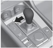
The gear position can be switched manually in manual shift mode. The manual shift mode indication and the gear position are displayed in the instrument cluster.
