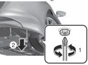
6. Turn the socket and bulb assembly counterclockwise and remove it.
