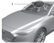
1. Forward Sensing Camera (FSC)
