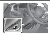
2. Adjust the steering wheel to the appropriate position.
