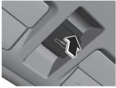
3. Press the tilt/slide switch forward.
