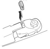
3. Raise the wiper arm and rotate the wiper blade to the right until it unlocks, then remove the blade.
