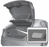
The luggage compartment lights turn on. When the liftgate is closed, the luggage compartment lights turn off.
