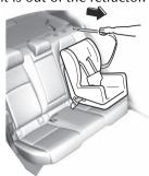
6. Push the child-restraint system firmly into the vehicle seat. Be sure the belt retracts as snugly as possible. A clicking noise from the retractor will be heard during retraction if the system is in the automatic locking mode. If the belt does not lock the seat down tight, repeat this step.
