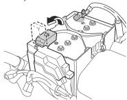
3. Turn off the booster vehicle's engine and connect the jumper cables in the following order.
