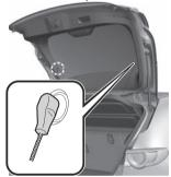
2. Press the luggage compartment cover upward from near the pins and remove the luggage compartment cover from the pins.
