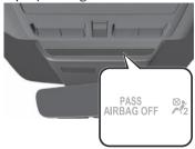
If the front passenger weight sensors are normal, the indicator light illuminates when the vehicle power is switched ON. The light turns off after a few seconds. Then, the indicator light illuminates or is off under the following conditions:
