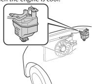
If it is at or near the LOW position, add enough coolant to the coolant reservoir to provide freezing and corrosion protection and to bring the level to FULL.
