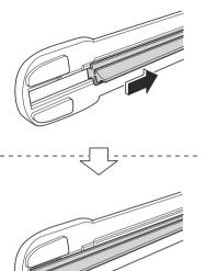
8. Make sure that the blade rubber is correctly installed to the blade holder.
