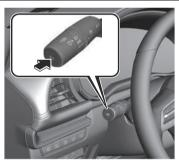
When the HBC is canceled, the HBC indicator light (green) hin the instrument cluster turns off. Press the HBC switch again to make the HBC operable.
