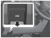
Insert your hand into the hood opening, slide the latch lever in the direction of the arrow as shown in the illustration, and lift up the hood.
