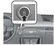
The engine starts and the KEY indicator light (green) and in the instrument cluster turns off.
