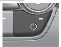
Switches the climate control system on and off.
