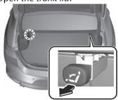
3. Open a rear door and fold the rear seat forward.
