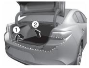
2. Turn the spare tire hold-down bolt counterclockwise and remove the spare tire.
