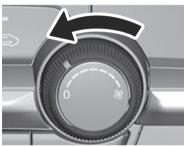
This dial allows variable fan speeds. The airflow amount can be adjusted to 7 levels.
