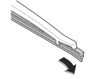
5. Remove the metal stiffeners from the blade rubber and install them in the new blade rubber.
