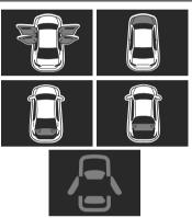
The light turns on if any door/trunk lid/liftgate/hood is not closed securely.
