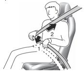
6. The belt should not touch the neck, jaw, or face and it should pass over the shoulder.
