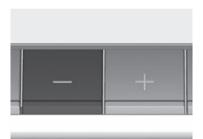
The airflow amount changes each time the switch is pressed. The airflow amount is indicated on the display. The airflow amount can be adjusted to 7 levels.
