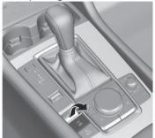
The brakes are applied and the vehicle can be decelerated/stopped. A sound is activated when the brake is applied and when the EPB switch is released, the brake will be released and the sound stops.
