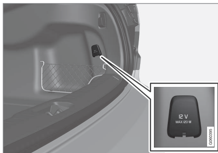
12 V outlet in trunk/cargo compartment*.
