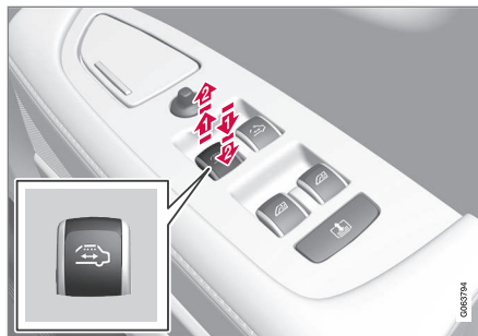
Sun curtain control.
